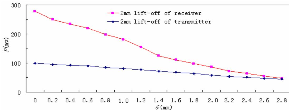
Fig.6 results of 2mm lift-off for transducers
