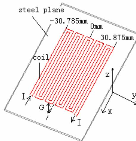
Fig.1 sensor coil configuration
