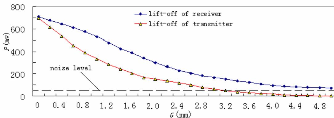
Fig.5 received signal at different lift-off values of transducers
