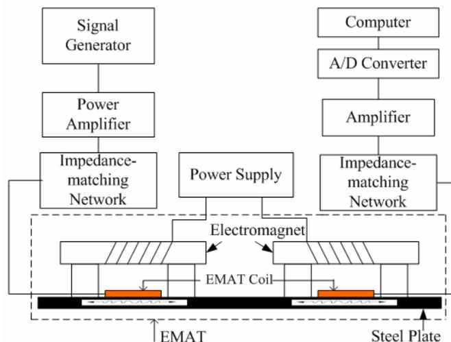
Fig. 4 block diagram of the experimental setup
