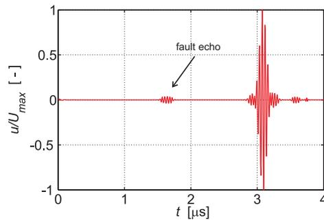
Fig. 5c. Filtered ultrasonic signal using dual filtering algorithm
