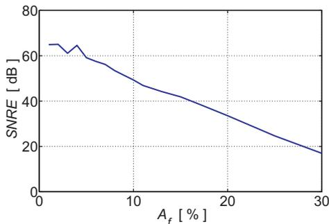
Fig.4a. Dual-filtering algorithm evaluation in terms of noise suppression
