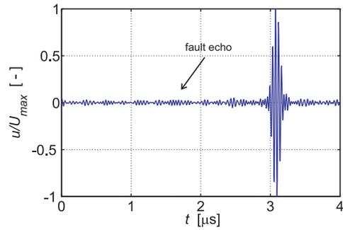
Fig.5b. Filtered ultrasonic signal using Wiener filter
