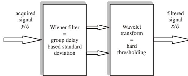
Fig. 3: Principal of dual filtering algorithm
