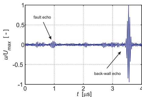
Fig.1: Simulated ultrasonic signal
