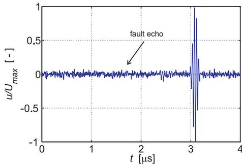
Fig.5a. Simulated ultrasonic signal with 2% fault echo amplitude
