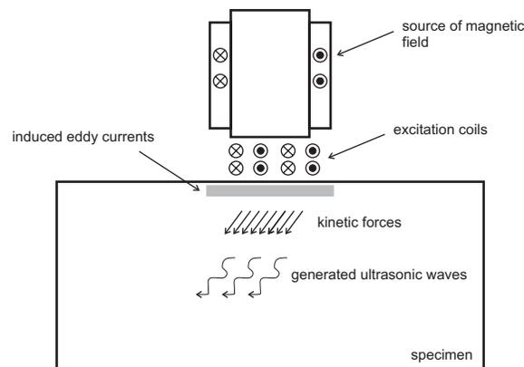
Fig. 1. Principal of ultrasonic wave generation using dual EMAT configuration
