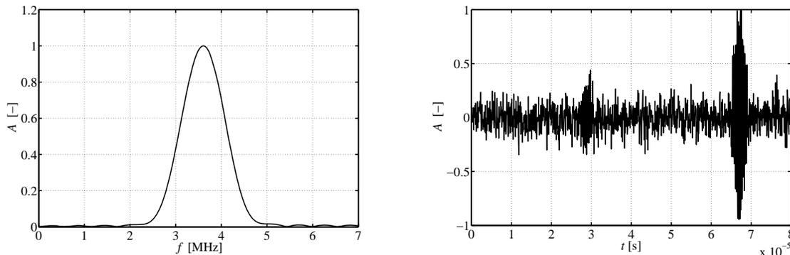
Fig. 4. Frequency response (left) and simulated EMAT signal (right)
