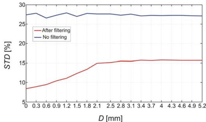
Fig. 8. Evaluation of BSS method on EMAT signals
