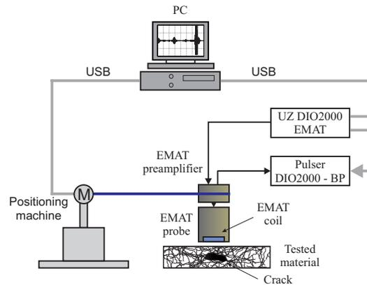
Fig.6. Full EMAT acquisition system
