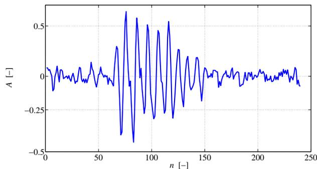
Fig. 2. Acquired EMAT signal on calibration gauge K1
