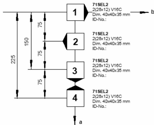
Figure 5. Probe configuration for Surge line examination
