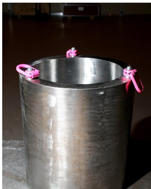
Figure 6. Surge line open test block
