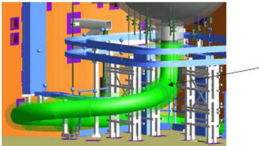
Figure 2. Location of one of the circumferential welds (“SL\_20”) on the surge line upper part
