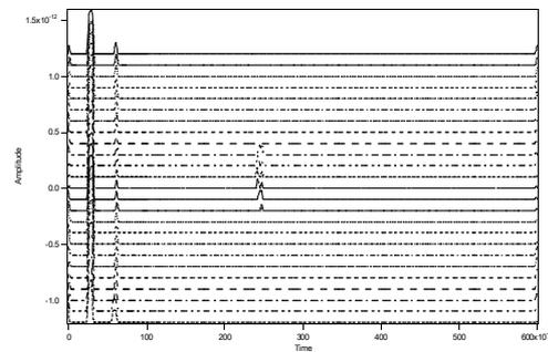
Figure 7. B-scan diagram of the energy-time relations of a concrete specimen with single rectangular defect within a frequency band of center frequency  $12.5\text{KHz}$  and half bandwidth  $\Delta f$  equal to  $2\text{KHz}$ .
