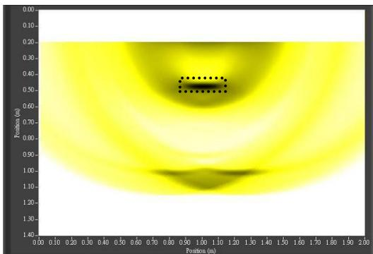
Figure 6. A SAFT image generated from time domain signals.
