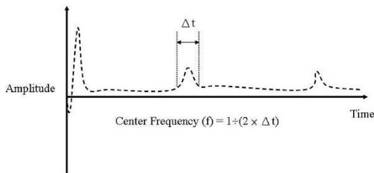
Figure 2. A typical signal in time domain.
