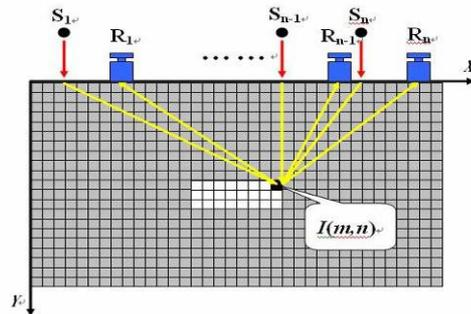
Figure 1. Implementation of impact-and-receive operations and meshing of specimen for the image construction by SAFT.
