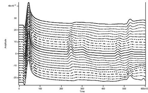
Figure 5. B-scan diagram of the measured signals in time domain of a concrete specimen with single rectangular defect.
