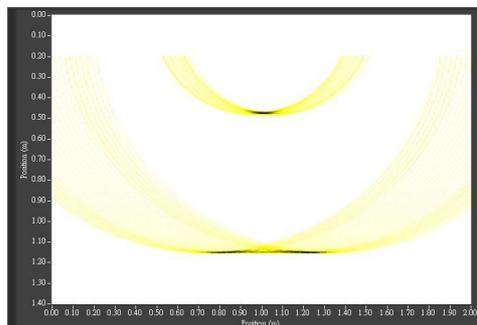
Figure 8. A SAFT image generated from responses of frequency energy varying in time.
