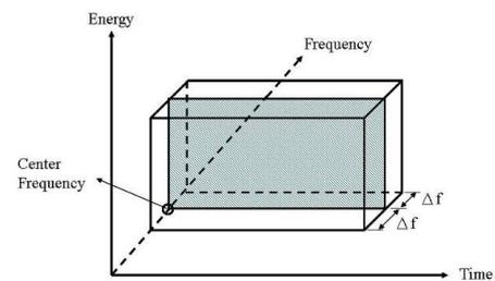
Figure 3. Relationship among time, frequency and energy of a signal after HHT.
