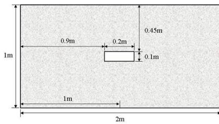
Figure 4. Dimensions of concrete specimen with a single rectangular shaped void defect.
