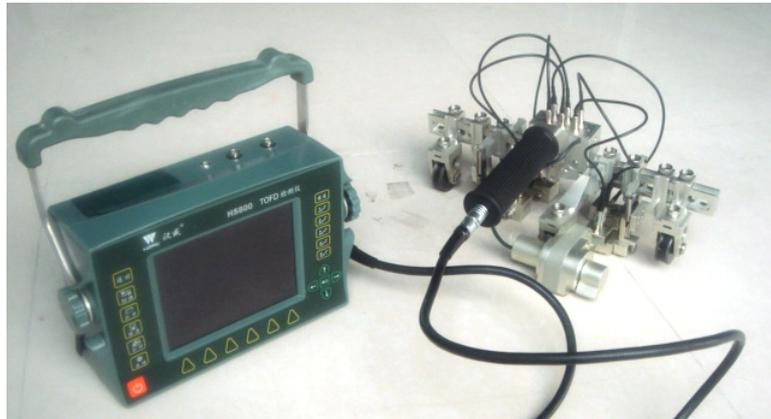
**Fig 2 HS800 TOFD ultrasonic testing instrument**
