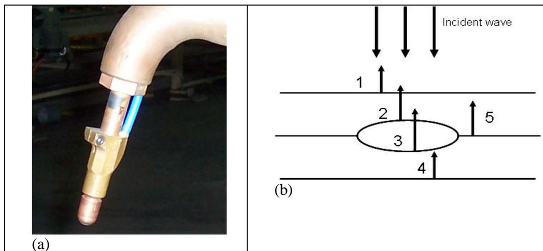
Figure 2. (a) – the ultrasonic wave penetrating the weld area; (b). the typical A-scan received from the weld.
