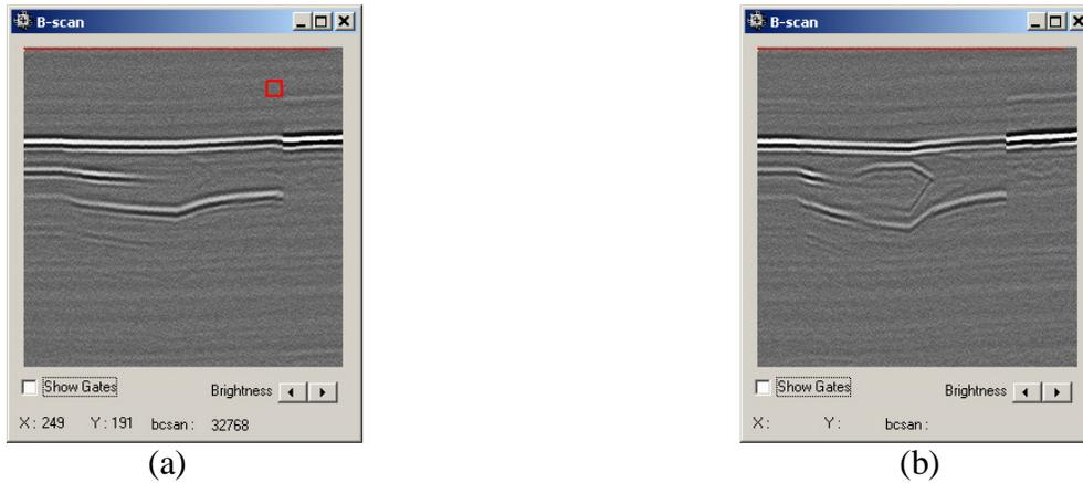
Figure 3. (a) – B-scan representing a stick weld; (b). the typical B-scan representing a good weld.
