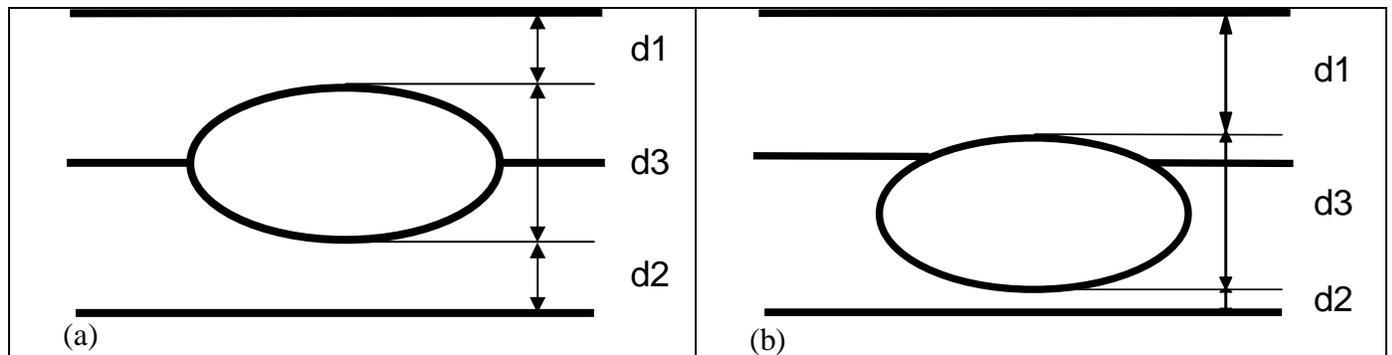
Figure 4. (a) – the symmetrical case of same-material, same-thickness weld; (b) – the non-symmetrical case, the nugget is shifted towards one of the welded plates making the joint weaker.
