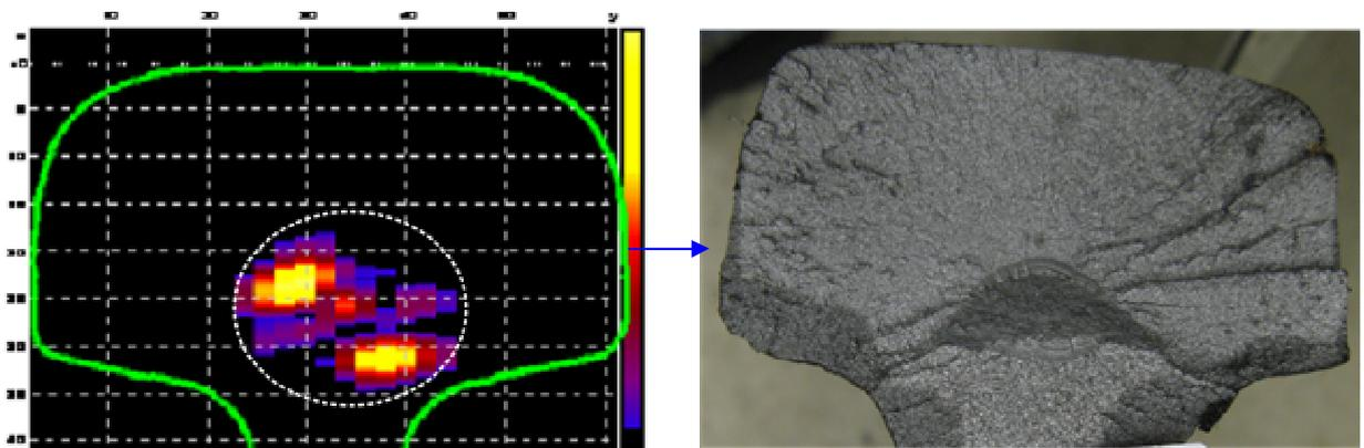
**Fig. 3 D-image (across the rail) of rail section with real flaw – transversal crack in the weld (left pane) and photo of fracture at the defected section (right pane)**
