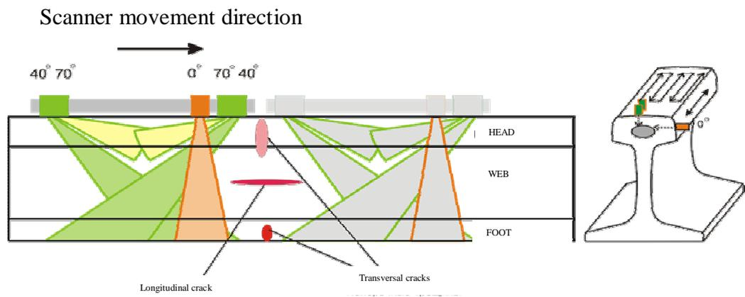
**Fig. 2. Inspection techniques scheme**
