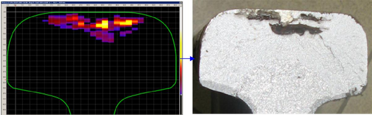
**Fig. 4 D-image (across the rail) of rail section with real flaws – horizontal exfoliations and progressive crack (left pane) and photo of fracture at the defected section (right pane)**
