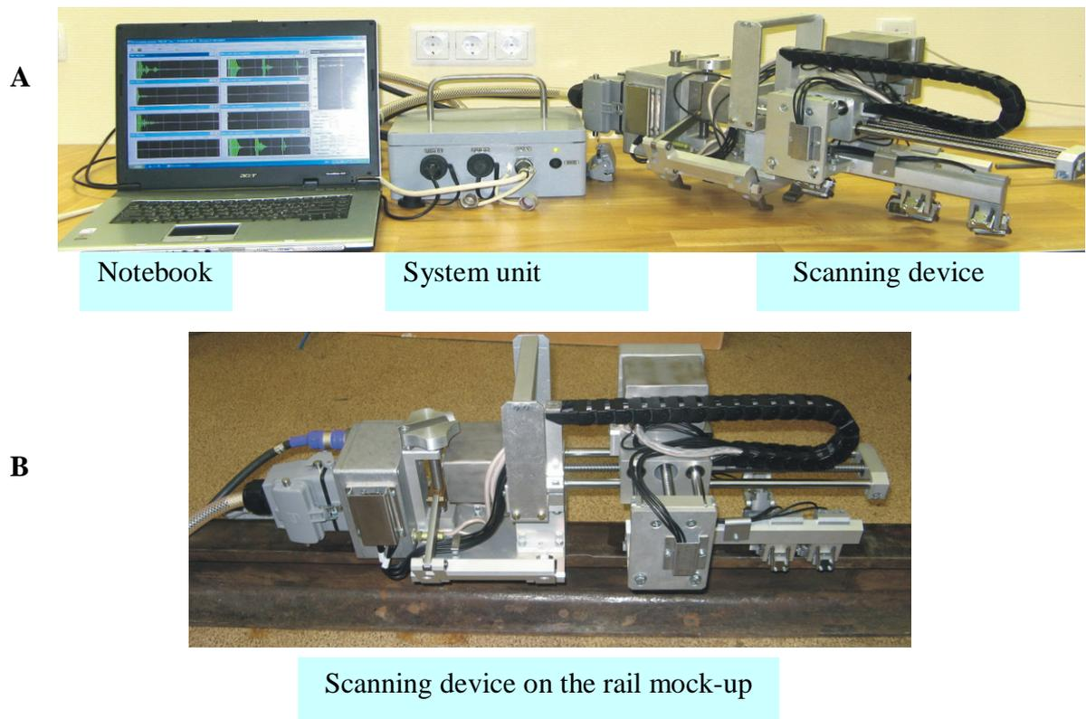
**Fig. 1. Acoustical holography system: A. Common view. B. Scanning device on the rail mock-up**
