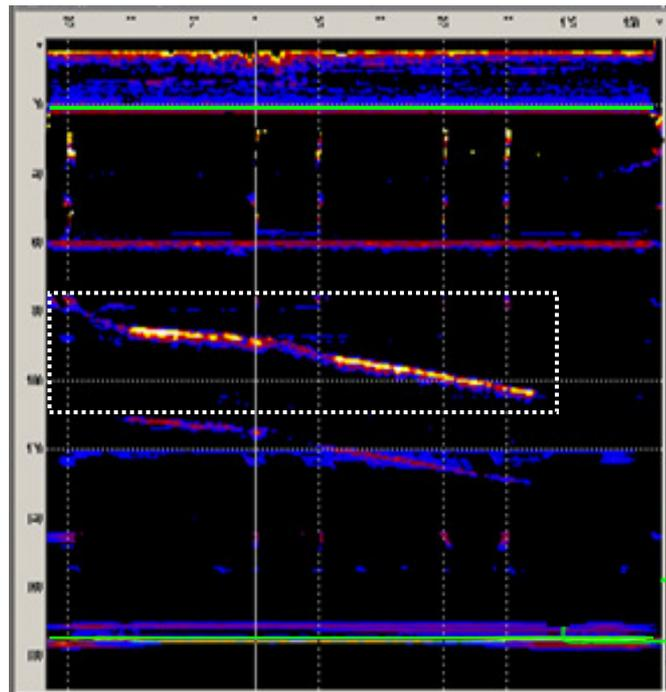
**Fig. 5. B-view (along the rail) of rail section with longitudinal horizontal exfoliation in web**
