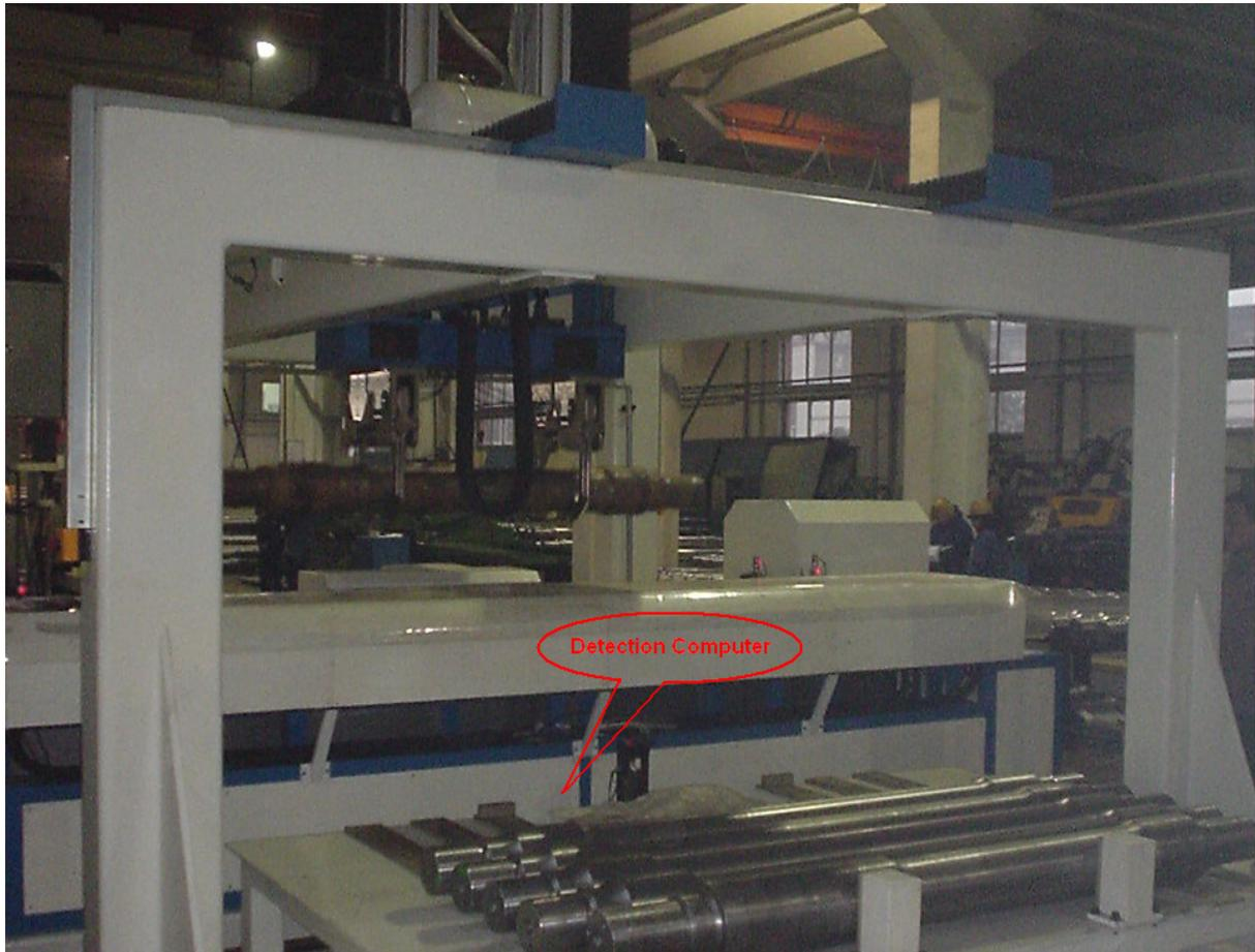
Figure 3. Axle automatic ultrasonic detection system
