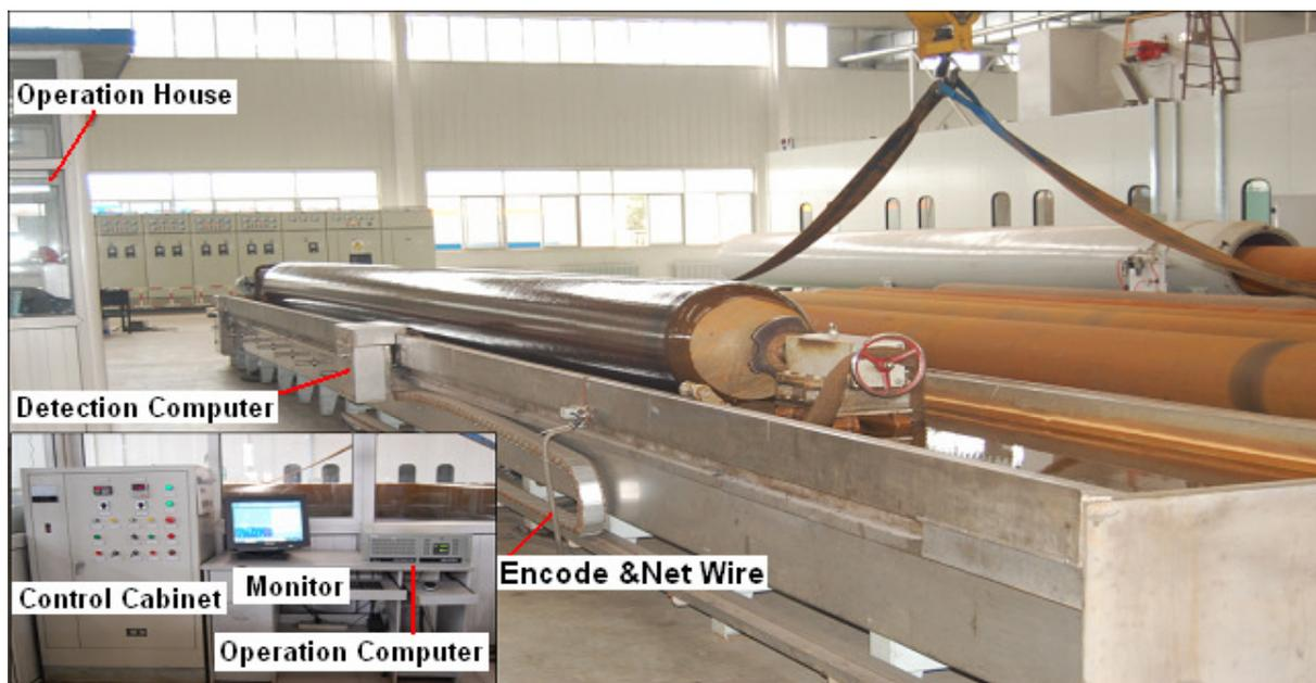
Figure 2. Picture of entire steel pipe body inspection system
