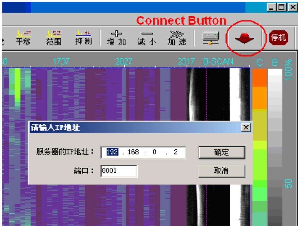
Figure 5. Axle automatic detection software interface relative to network transmission
