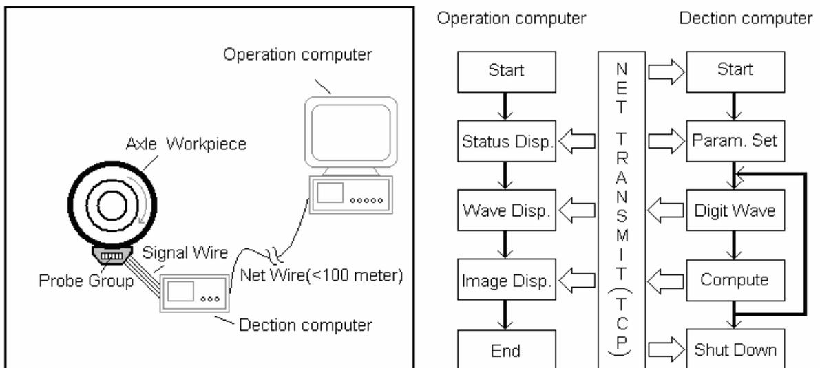
Figure 4. Schematic drawing of network transmission structure
