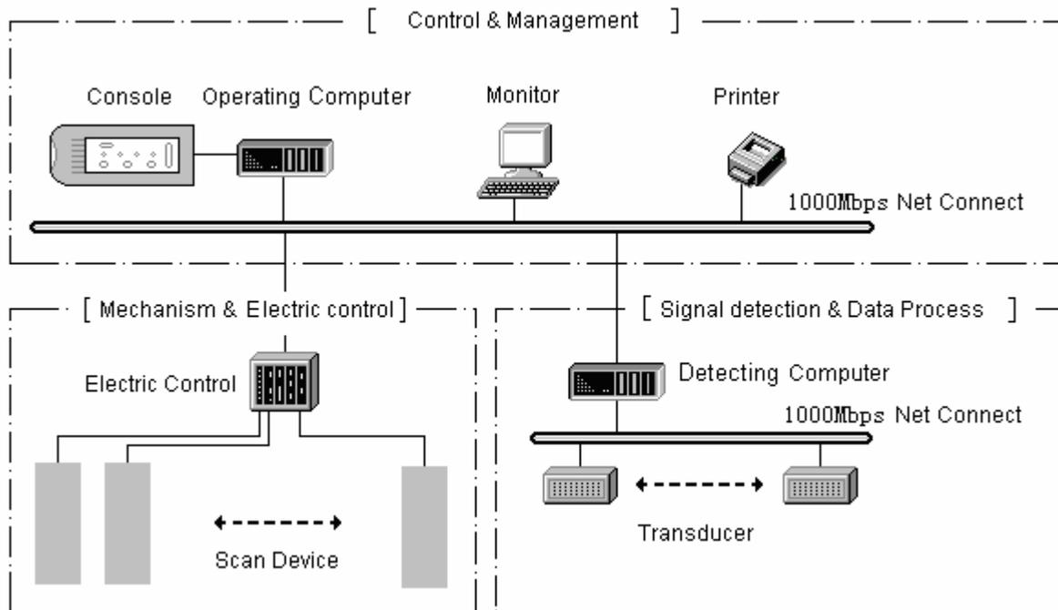
Figure 1. Schematic drawing of network transmission system structure
