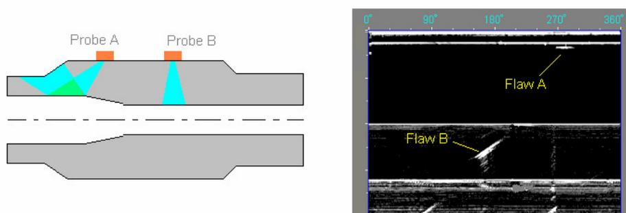
Figure 4. Ultrasonic automatic inspection for drill head:
