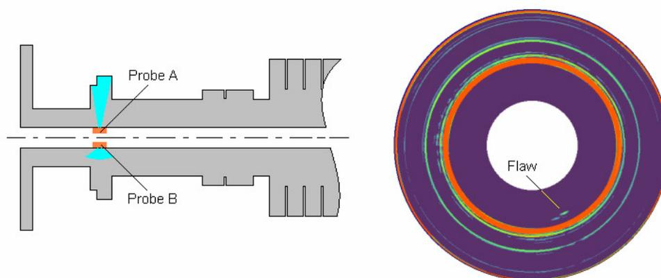
Figure 2. Ultrasonic automatic inspection for rotors center of turbine bores:
