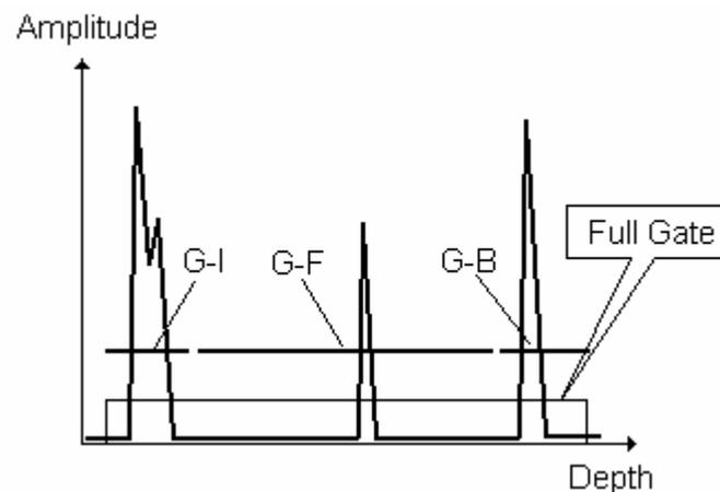
Figure 1. Full data acquisition gate
