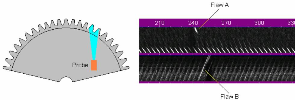
Figure 3. Ultrasonic automatic inspection of locomotive drive gear:
