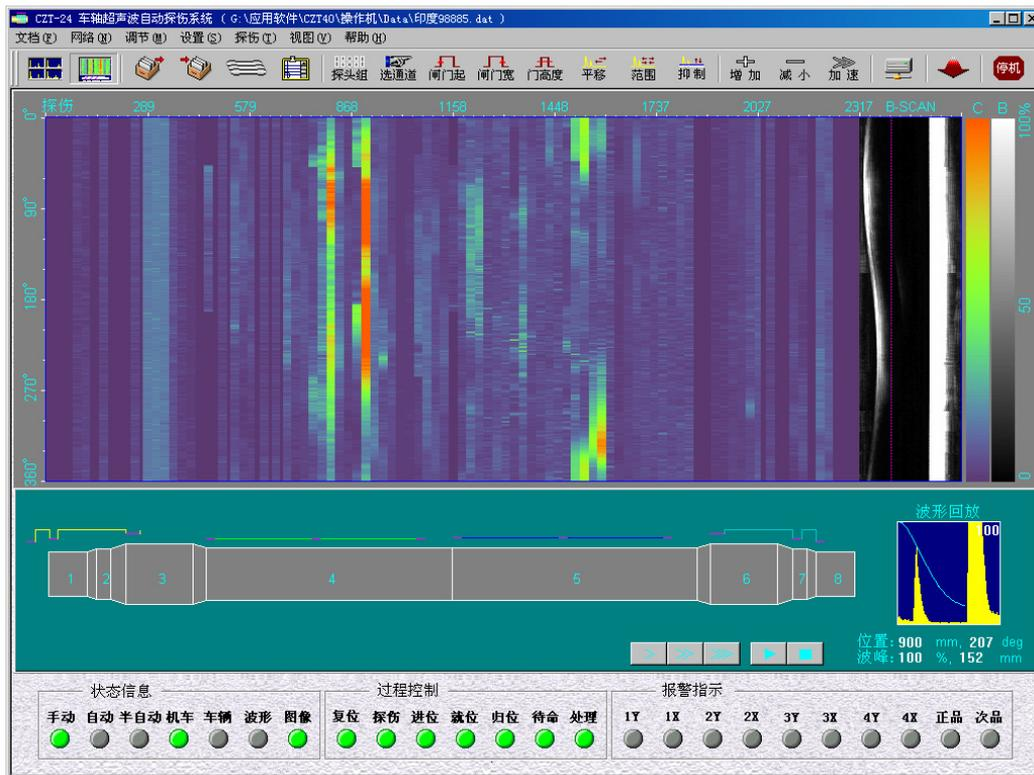
Figure 5. Automatic ultrasonic inspection image display for axle
