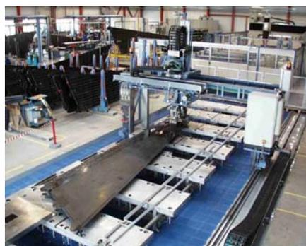
Figure 2 – Ultrasonic gantry system
