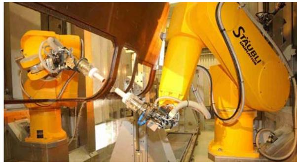
Figure 3 – Ultrasonic robotic system
