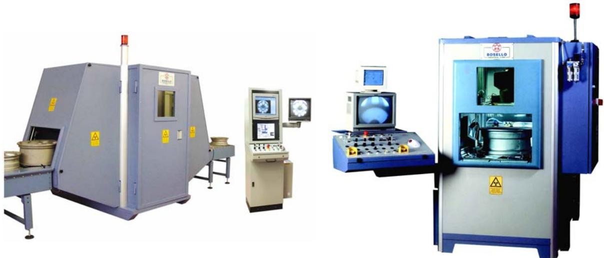
Figure 4 and figure 5 – Fully automatic wheel testing system with software of wheel recognition and automatic assessment.
