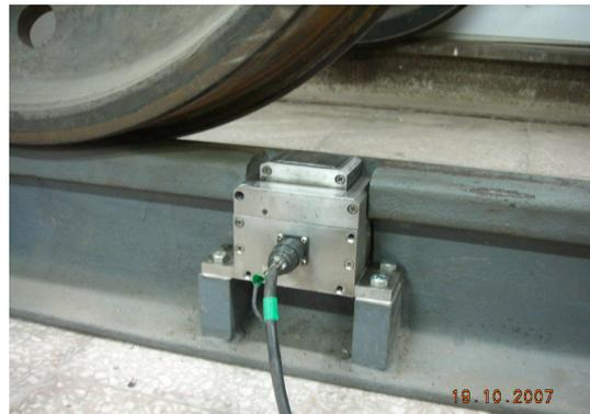
Fig. 6 EMAT is installed on rail
