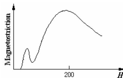
**Fig. 3 Relation between Magnetostriction and Field Strength**
