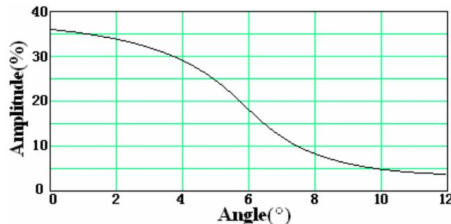
**Fig. 4 Sound Field Strength versus Half-Angle of Spread**
