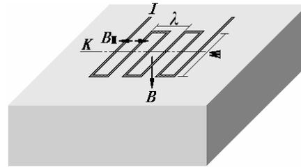
**Fig. 2 Principle of EMAT**
