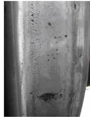
**Fig. 1 Fall-block on Wheel Tread**
