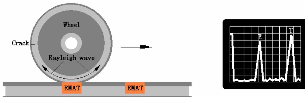
**Fig. 5 Transmission of Rayleigh Wave in Wheel Treads and Display**
