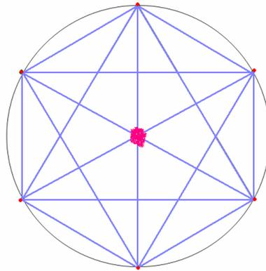
**Fig. 5** The guided wave ray paths in the tomography
