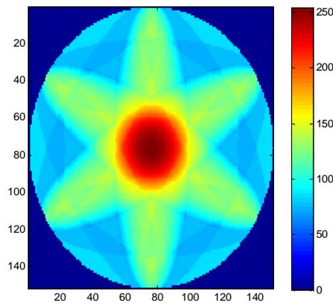
**Fig. 6 The tomography of V-notch located in the middle with 6 transducers**
