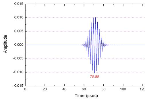
**Fig. 3 S0 Mode propagation result**
