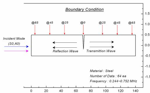
**Fig. 1 BEM model of a plate with V-notch**
