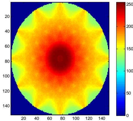
**Fig. 7 The tomography of V-notch located in the middle with 12 transducers**
