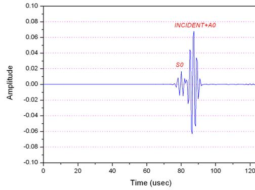
**Fig. 2 The reflected time domain signal for S0 mode incidence at 45mm from defect location**
