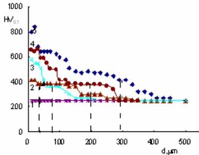
Fig. 1. Micro-hardness distribution in the specimen cross section
