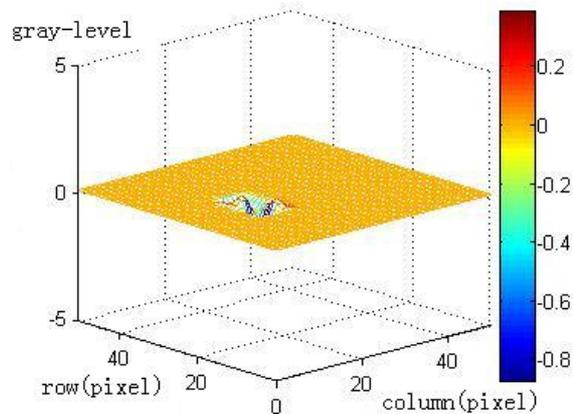
Fig. 7 3-D gray-level distribution of false defect after background subtraction
