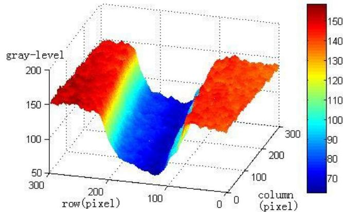
Fig. 5 3-D gray-level distribution of background image by partial surface reconstruction
