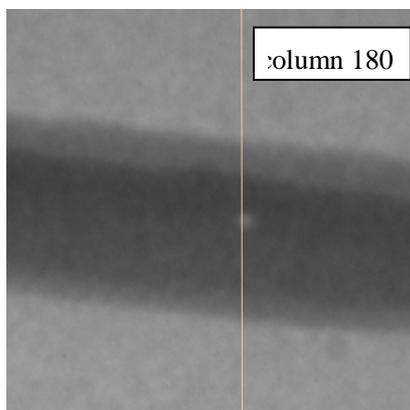
Fig. 1 Real-time X-ray image of double-side weld
