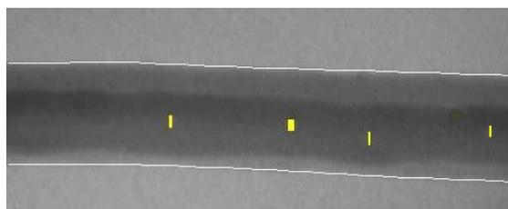
Fig.5 defect segmentation result of gray-level wave analysis
