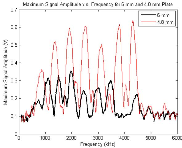
Figure 3. Maximum RF amplitude as a function of frequency for two stainless steel plates of different uniform thicknesses.
