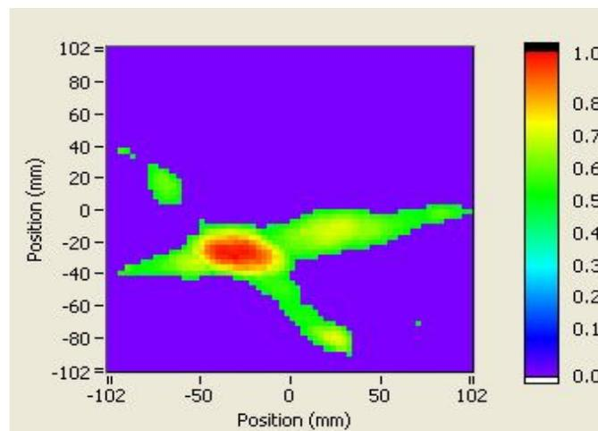
Figure 1. Tomogram taken using a 16-sensor array on a steel pipe elbow. See [4] for more details.
