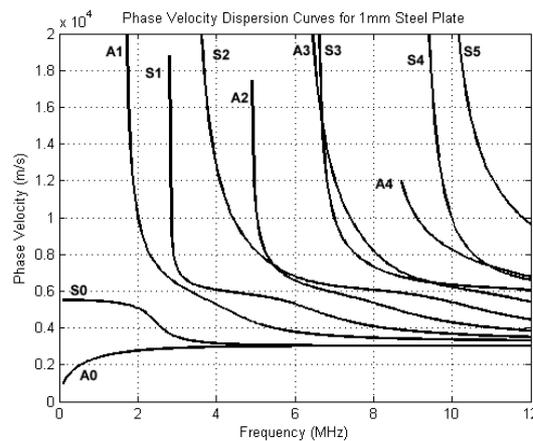
Figure 2. Phase velocity dispersion curves for a 1 mm steel plate.
