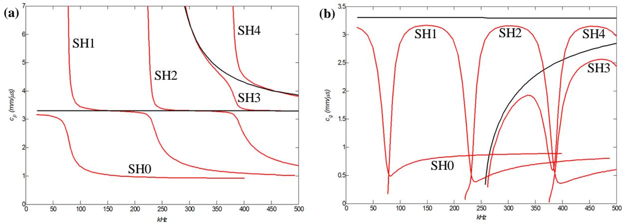
Figure 1: Phase (a) and group (b) velocity dispersion curves for a 20''-diameter schedule 10 pipe with a 3mm-thick coal-tar wrap coating. Black lines correspond to the bare pipe case and are shown for comparison.
