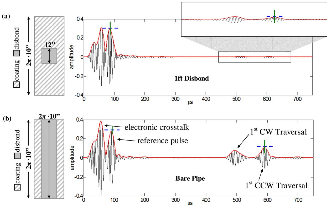
Figure 3: Ultrasonic waveforms obtained from a 20"-diameter schedule 10 pipe with a coal-tar wrap coating with a (a) 1ft. disbond and for a (b) bare pipe. The SH1 modes was used at a frequency of 130kHz.
