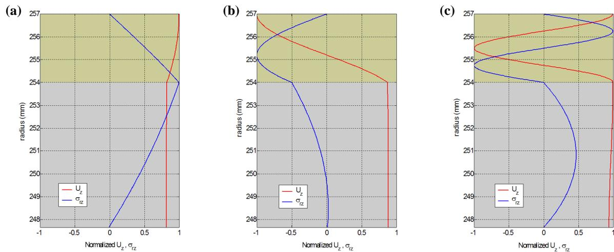
Figure 2: Particle displacement and shear stress distributions for (a) SH0 at 30kHz, (b) SH1 at 130kHz, and (c) SH2 at 312kHz.
