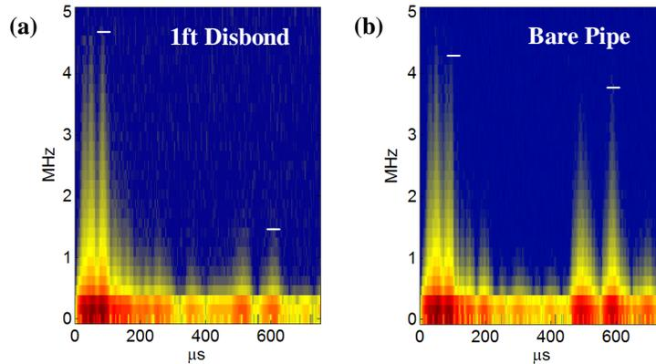
Figure 4: STFTs of RF-waveforms for a (a) 1ft disbond and a (b) bare pipe. A 64-point Hanning window with 32-point overlap was used.
