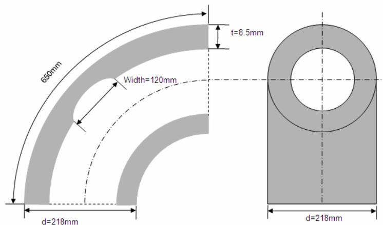
Figure 2. Shape of defects in 8.5mm thick elbows
