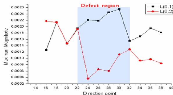
Figure 6. Maximum Magnitude using line scan technique on defect region.
