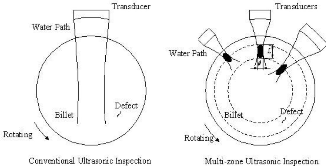
Figure 1. Conventional and multi-zone longitudinal wave inspections
