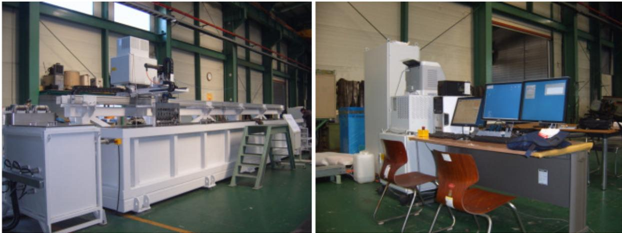
Figure 2. Overview of immersion multi-zone ultrasonic inspection system
