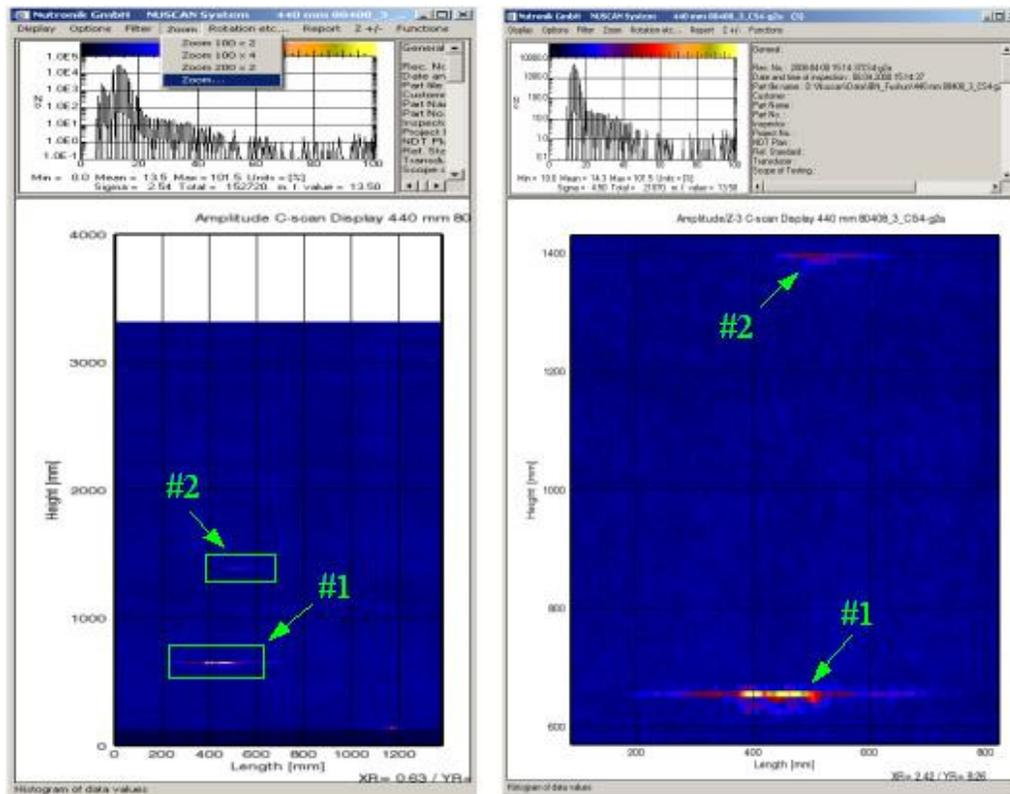
Figure 11. C-Scan images of billet with diameter 440mm
