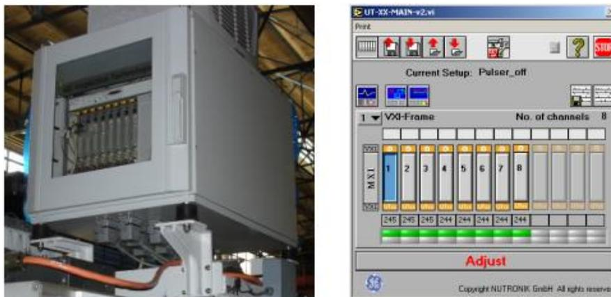
Figure 6. Eight-channel parallel digital ultrasonic instrument, UTxx71.00
