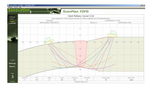
The software calculates the nominal Probe Centre Separation (PCS), probe characteristics (Frequency, diameter et cetera) and inspection coverage. The inspection coverage is displayed by the beam spread and the longitudinal wave loci for the back wall
