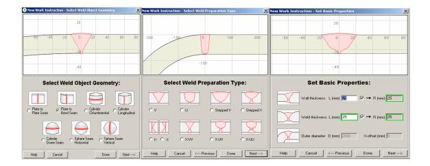
Once the geometry has been established, the software suggests a basic examination strategy which is based upon experience and the requirements of the standard chosen. The result can now be further optimised for the specific configuration, because the software immediately has processed the set up and calculated a number of key parameters which are to an extent visualized on the ScanPlan<sup>®</sup> display.
