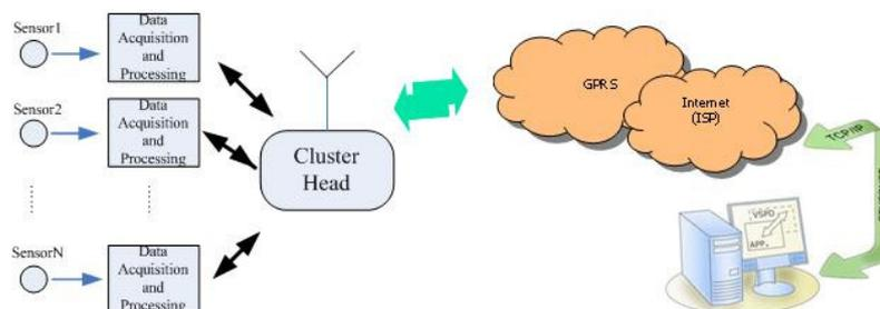
Figure 1. Structure health tele-monitoring system
