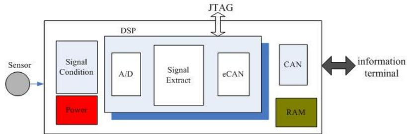
Figure 2. Hardware module frame of the signal acquisition and processing node
