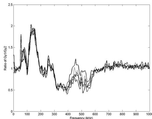
Figure 5. The ratios of  $G_{y1}/G_{y2}$  for various leak sizes of valve 2 inch.
