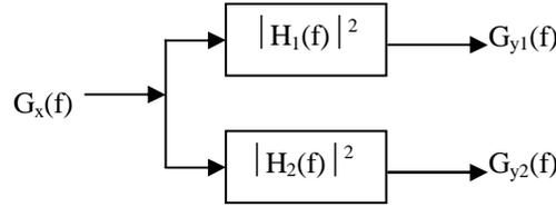
Figure 1. Different signal propagation paths with a common input
