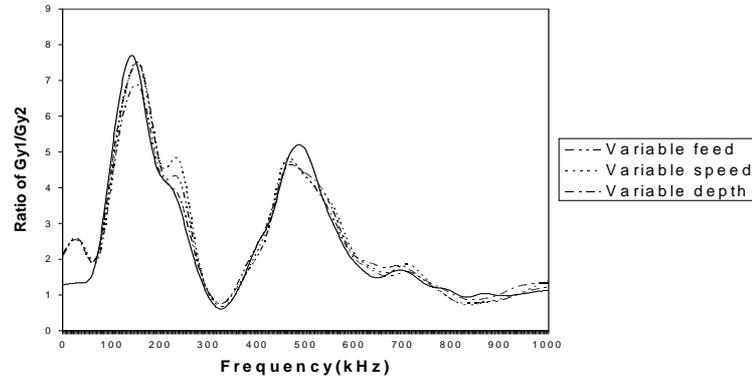
Figure 4. The ratios of  $G_{y1}/G_{y2}$  for the three sets of machining tests.
