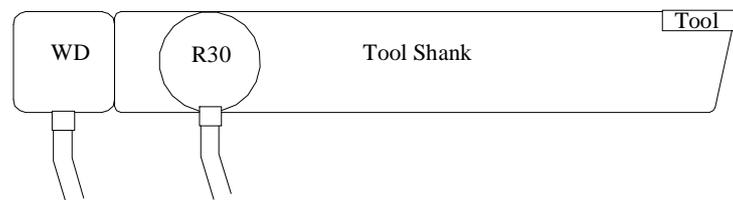
Figure 2. Two AE sensors (WD and R30) on the tool holder
