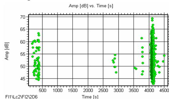
Figure 3 Distributive AE amplitudes vs. time
