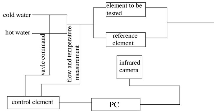
Fig. 3. Test-bed diagram
