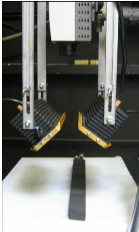
Fig. 5. The ARGUS set-up for pulsed IR thermography<sup>[17]</sup>
