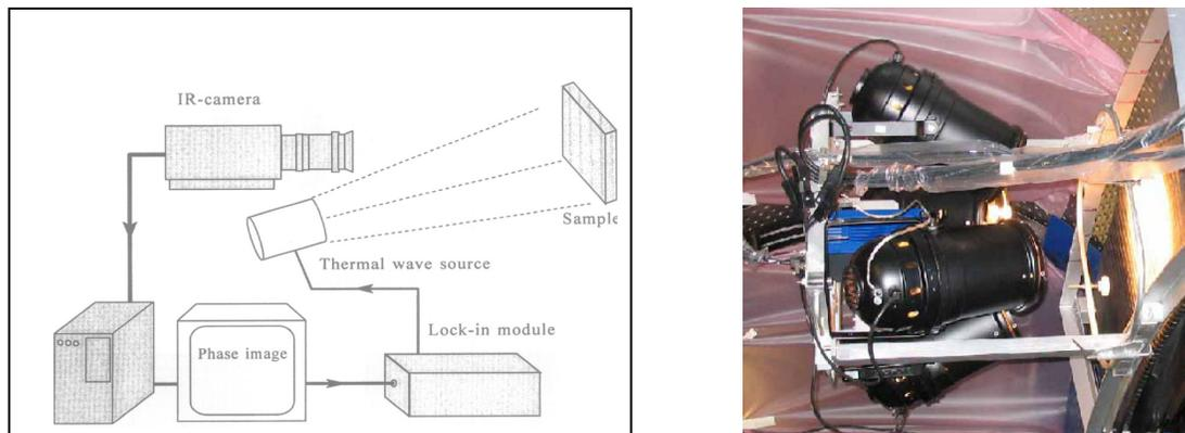
Fig. 4. Left: principle schematic of lock-in thermography<sup>[12]</sup>; right: an in-filed lock-in<sup>[15]</sup>
