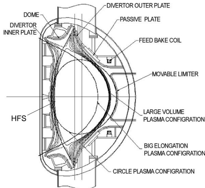
Fig. 1. Elevation view of EAST PFCs<sup>[1]</sup>.
