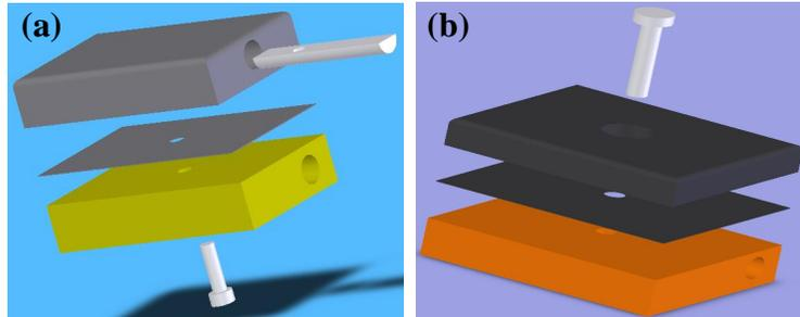
Fig. 2. Schematic figures of two types of PFC modules with active cooling, (a) for areas of high heat load (divertor), and (b) for areas of low heat load (HFS, passive plate, etc.), expecting to withstand heat fluxes less than 1 and 3 MW/m<sup>2</sup>, respectively.
