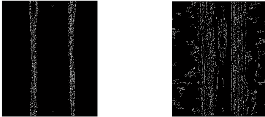
(a) Sobel operator edge detection (b) Canny operator edge detection
