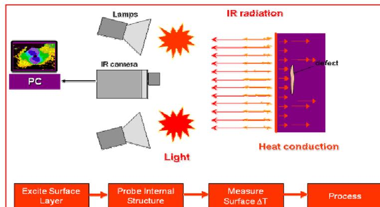
Figure 1. The operating principle of the Pulsed heating thermal wave NDT
