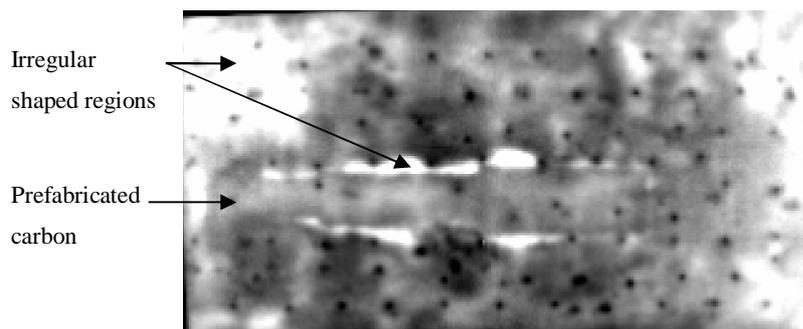
Figure 3.Original thermal image obtained by the thermal wave NDT
