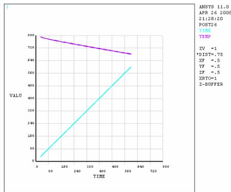
Fig.8. The curves of cooling on heating plane and rise in temperature on surface of the model
