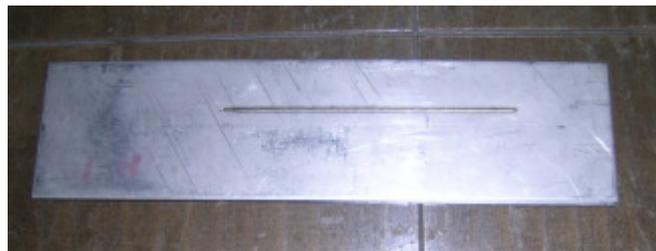
Fig. 1 the steel plate with welded joint
