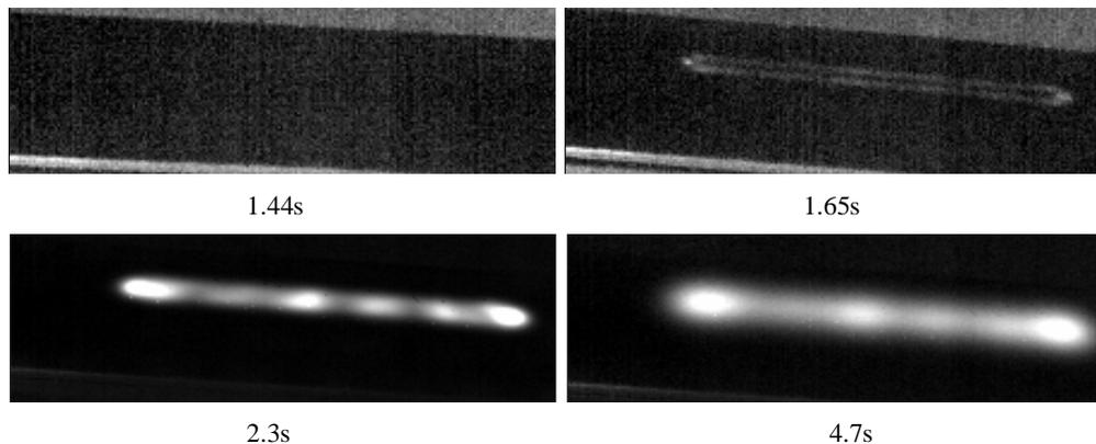
Fig. 3 Ultrasonic-heated thermal wave images of the steel plate with welded joint sample.
