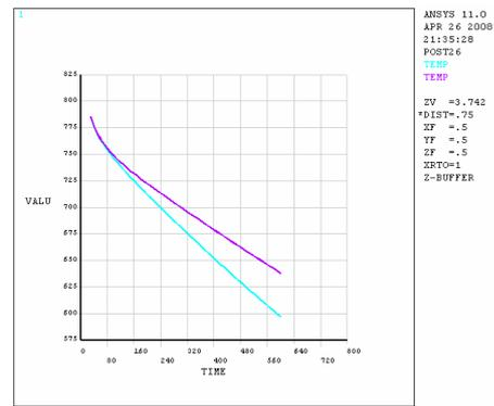
Fig.9. The curves of cooling about different point on surface of the model
