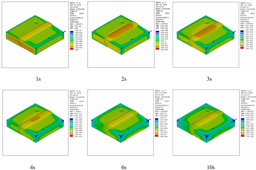
Fig.6.The equivalent diagram of temperature field profile about the model
