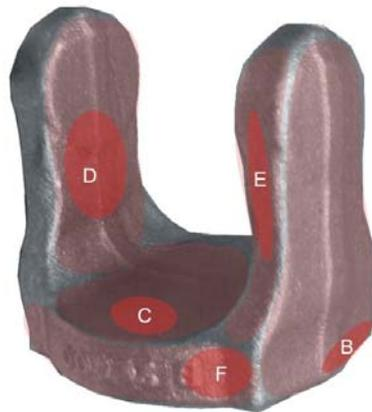
Fig. 7: Component with markings at typical defect positions
