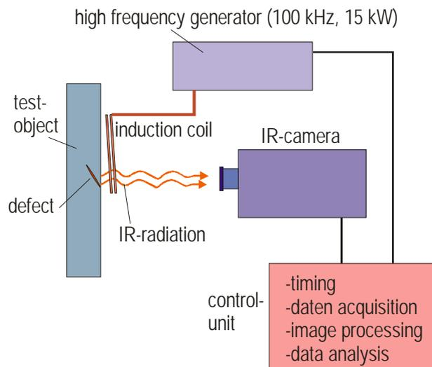
Fig. 1: Scheme of a set-up for induction thermography
