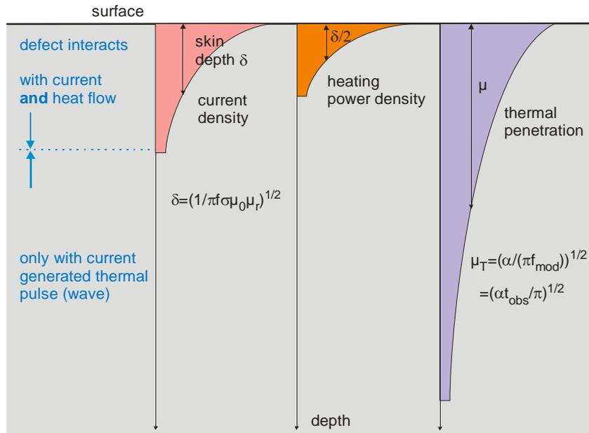
Fig. 2: Characteristic lengths for defect detection
