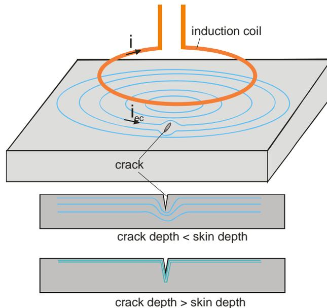
Fig. 3: Scheme of a set-up for induction thermography
