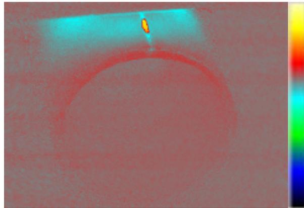
Fig. 6: Crack in a small automotive component
