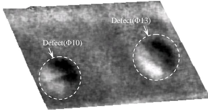
Figure 3. 2D imaging in the area with simulated defects
