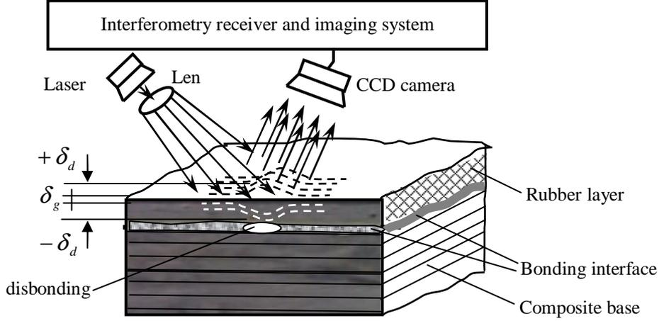
Figure 1. Illustration of the rubber-composite bonding structure and testing principle
