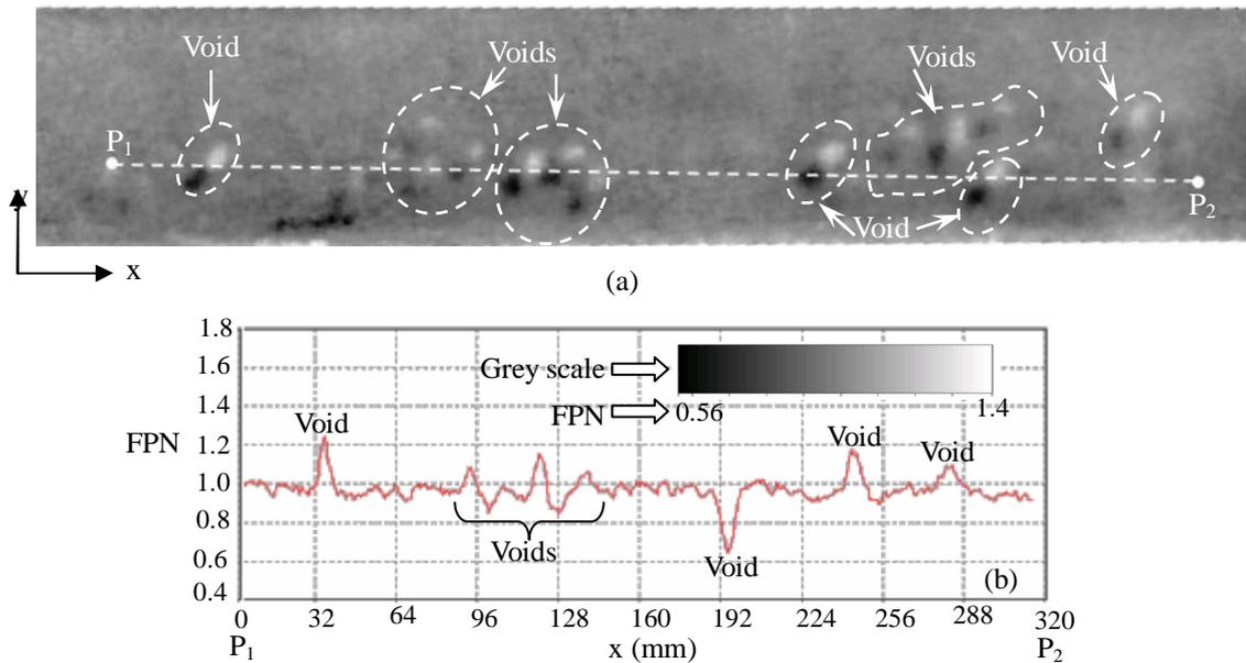
Figure 4. The shearographic imaging results from a practical rubber-composite bonding component. (a) 2D image, (b) FPN distribution corresponding to the marked position by the white line P<sub>1</sub>-P<sub>2</sub> in (a)
