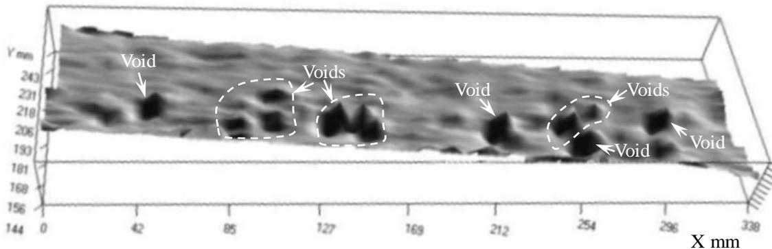
Figure 5. 3D imaging results of the rubber-composite bonding component
