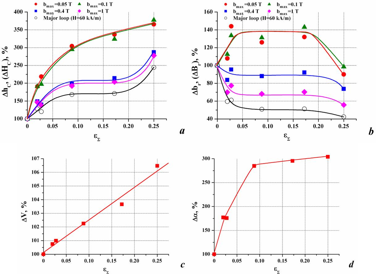
Fig. 1. Relative change of the coercive force (a), residual magnetic induction (b), the propagation velocity of a longitudinal acoustic wave (c) and the readings of the eddy-current instrument (d) as dependent on the accumulated plastic strain for the steel under study. The values of the physical characteristics for the steel in the initial annealed state are taken to be 100% (see the table).
