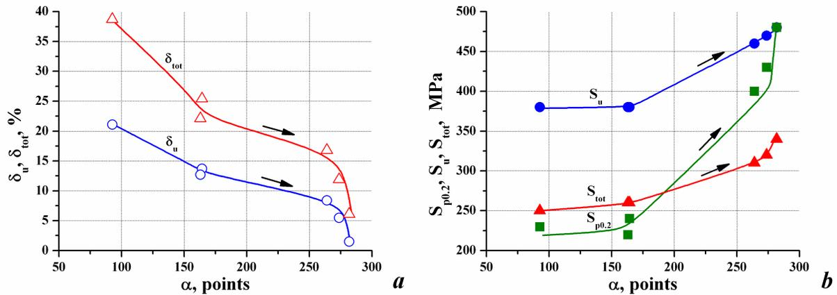
Figure 2. Correlations between the residual (after cyclic loading) strength and plasticity properties of the steel under study and the readings of the eddy-current instrument. The arrows show an increase in the number of loading cycles (accumulated plastic deformation).
