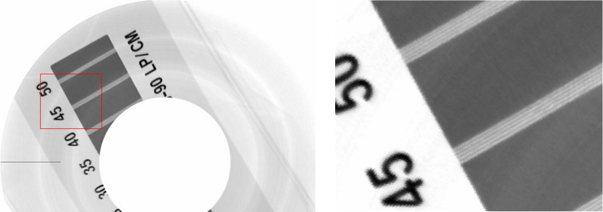
Fig.3 the resolution test card image
