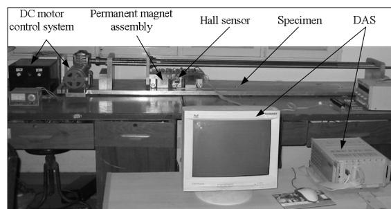
Figure 4. Photograph of the MFL measurements system
