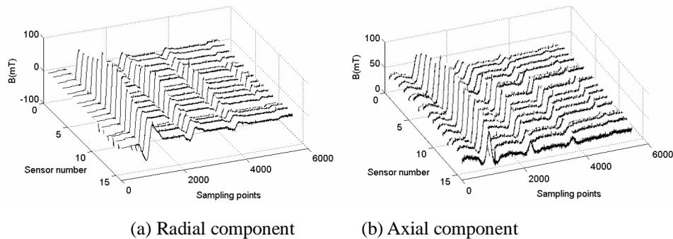
Figure 5. Plot of radial and axial component of magnetic flux density
