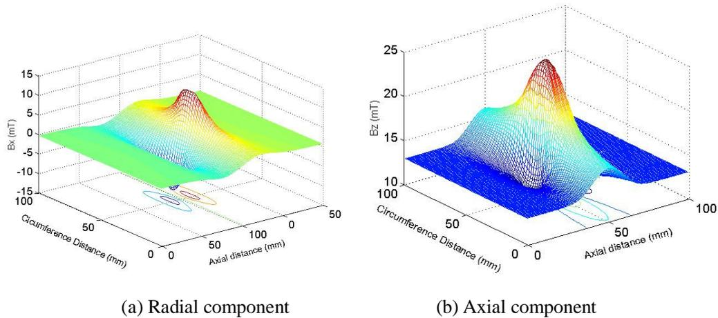
Figure 3. Surface plot of axial magnetic flux density
