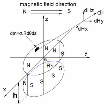
Figure 1. Defect dipole model
