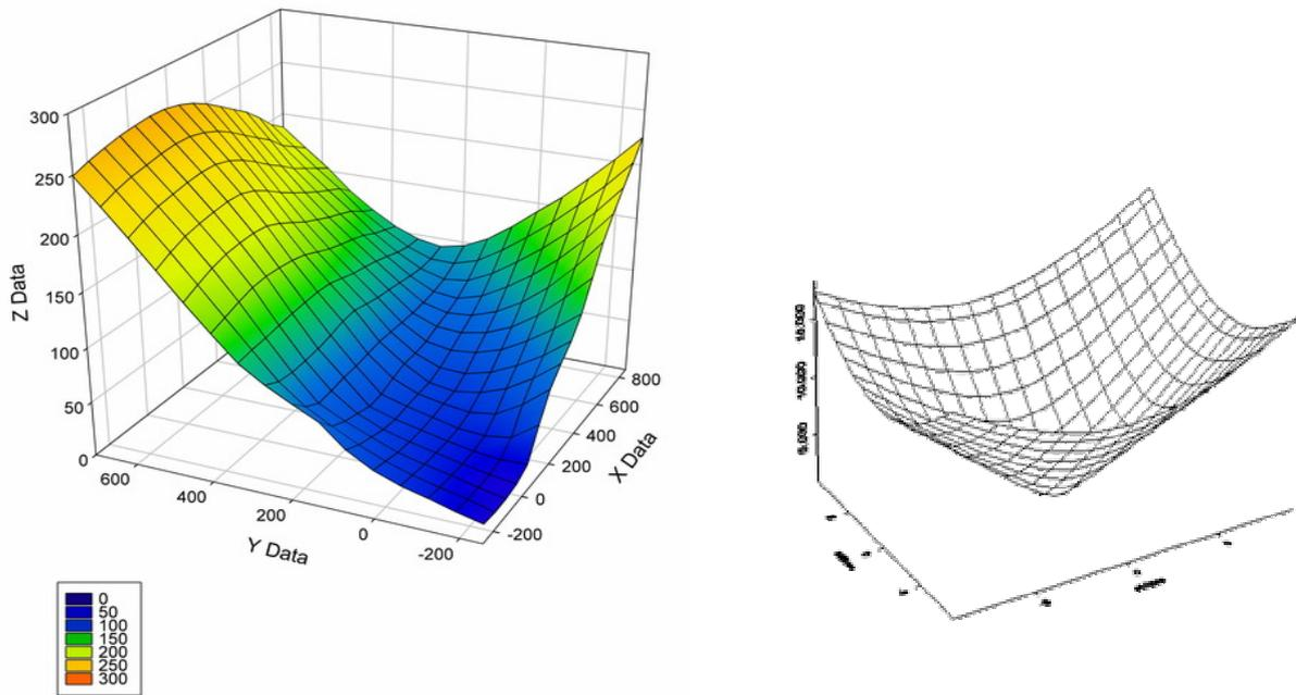
Fig.4. The surface  $p_M(\varepsilon_1, \varepsilon_2)$  for the “Mises BN signal” (left) for high strength alloy VNS-2 acquired from bi-axial stress tests. At right the regular Mises surface for the deformation in two directions is shown.
