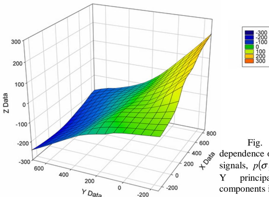
Fig. 3. Approximated dependence of the difference of BN signals,  $p(\sigma_1) - p(\sigma_2)$ , over X and Y principal elastic deformation components in low carbon steel.
