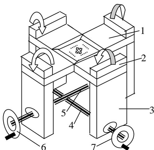
Fig. 2. Laboratory device for the cross-like specimen 1 testing by bi-axial bending: 2 – clamp; 3 – arm; 4,5 – driving screws; 6 – driving lever.
