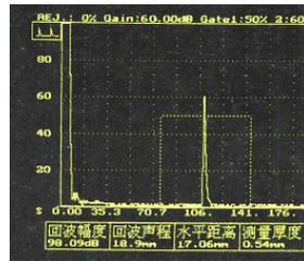
Fig.4 creeping wave signal
