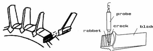
Fig.1 assembly position and detecting method of turbine blade
