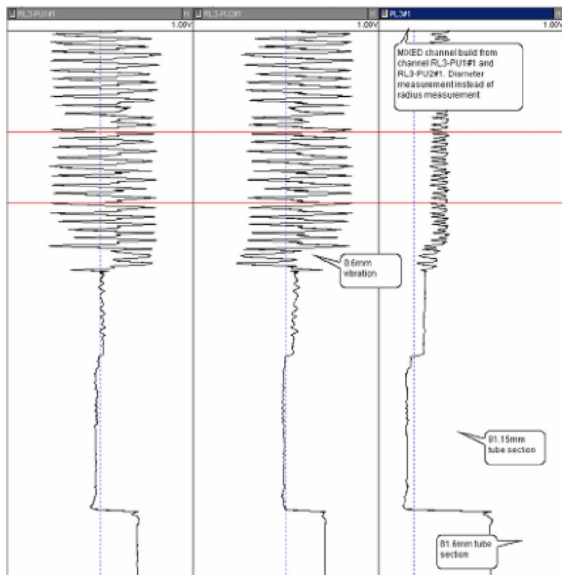
Figure 5. Noise reduction example; right strip chart is obtained by adding coil readings
