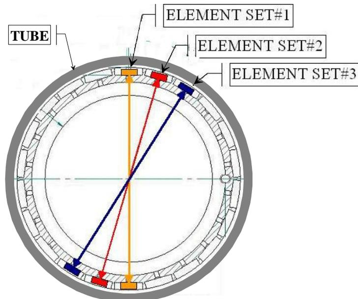
Figure 4. Set of opposite coils reading tube diameter
