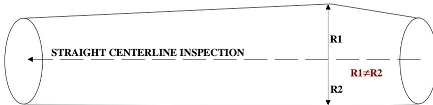
Figure 1. Straight centerline probe scan configuration
