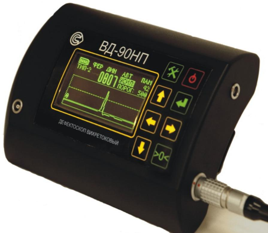
Figure 1. VD-90NP eddy current flaw detector. General view.
