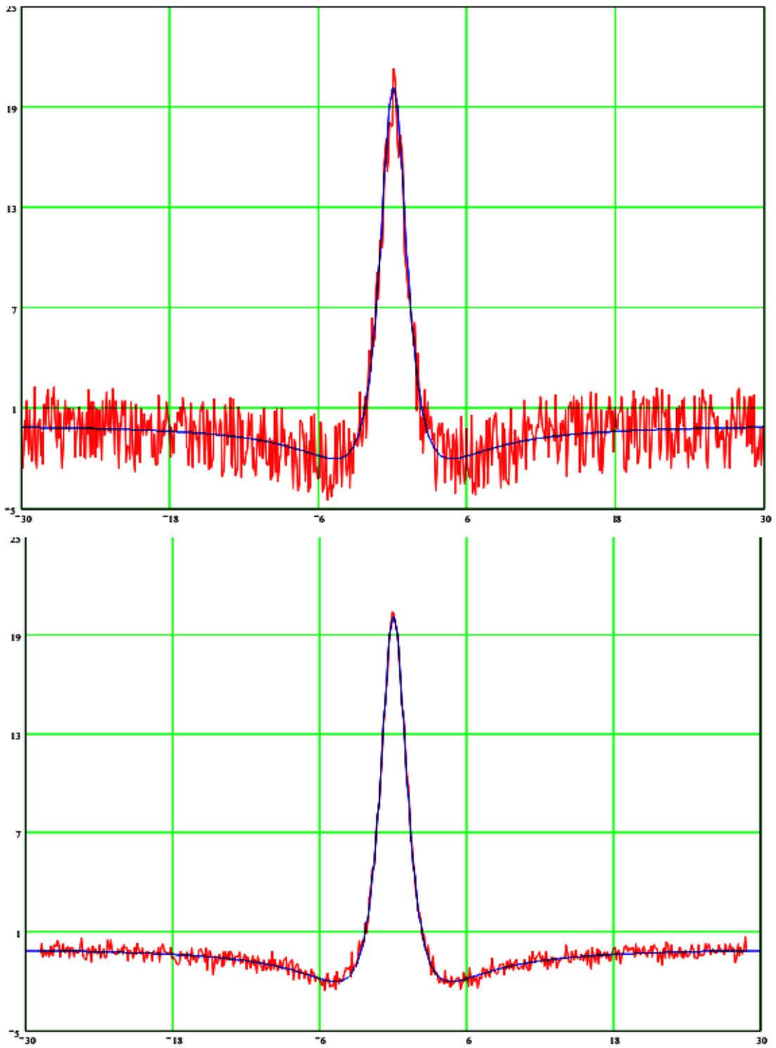
**Figure 5. Signal digitally filtered by a window function.**
