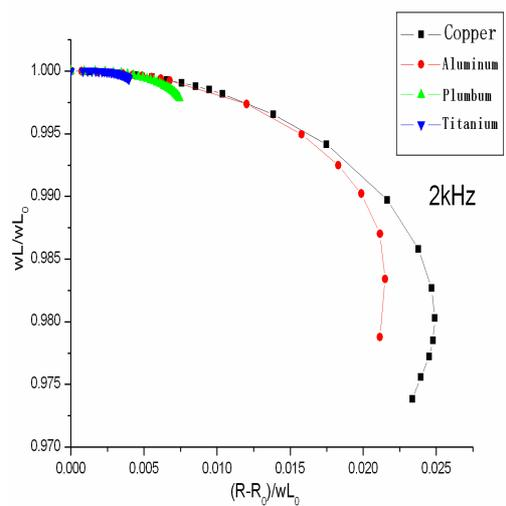
Figure 5-2 the impedance variation with changing substrate thickness under 2kHz
