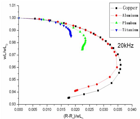
Figure 5-4 the impedance variation with changing substrate thickness under 20kHz
