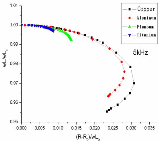
Figure 5-3 the impedance variation with changing substrate thickness under 5kHz
