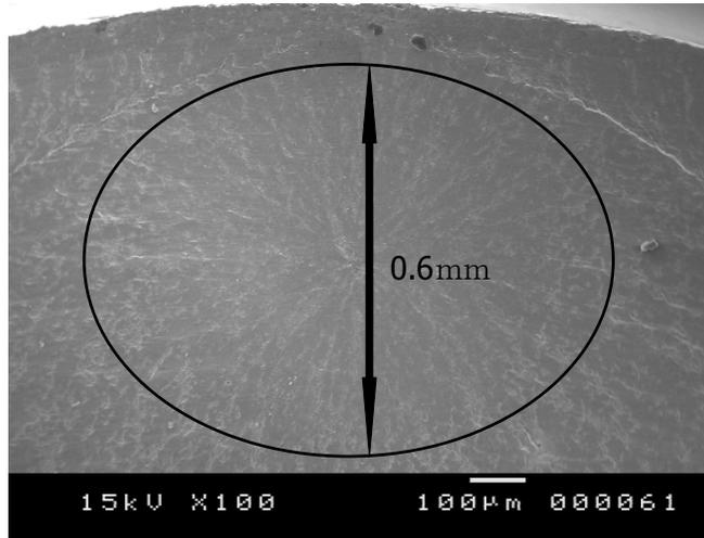
Figure 3 SEM micrograph of fatigue fracture surface of nitrided specimen
