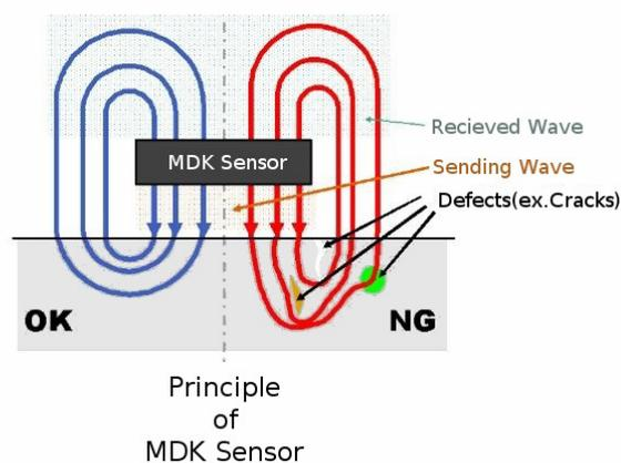
Figure A Principle of MDK Sensor
