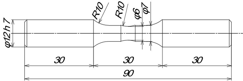
Fig.1 Shape and Dimension of Specimen
