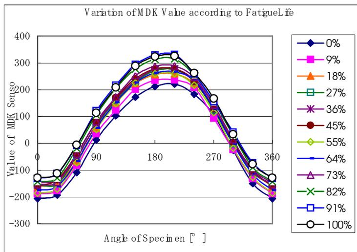
Fig.5 Variation of MDK Value according to Life Cycle (in Sectional Angle) [  $\sigma = 610\text{Mpa}$ ,  $N_f = 450000$  ]
