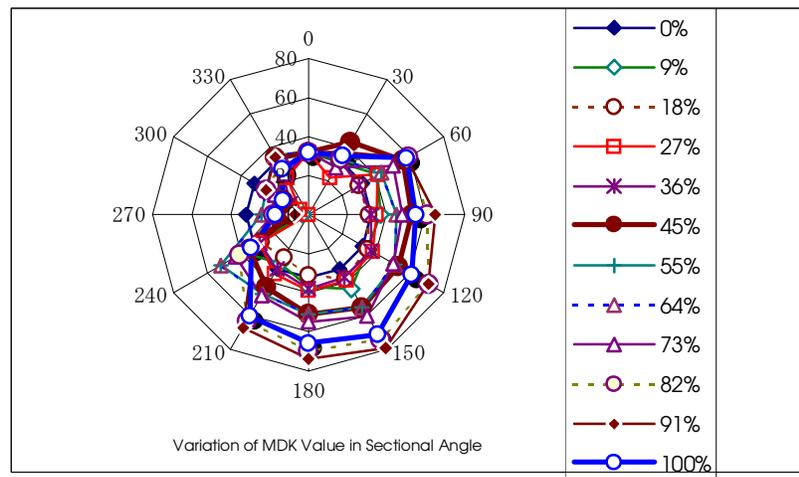
Fig.6 Variation of MDK Value in Sectional Area according to Fatigue Life
