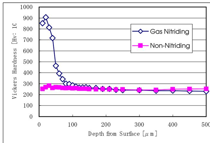
Fig. 2 Hardness of Gas Nitrided Steel (Hv: in Vickers Hardness Number)
