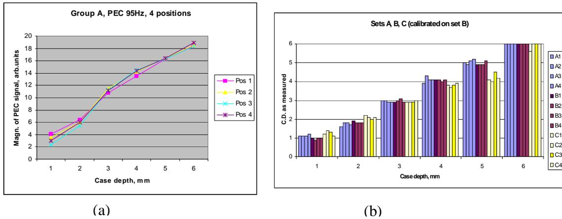
Fig. 7. Results obtained with the PEC system from one group of specimens (a) and three groups of specimens (b).
