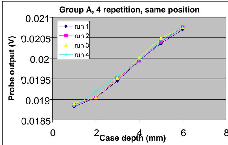
Fig. 4. Repeatability measurements of MFEC system on the same location of sample set A.
