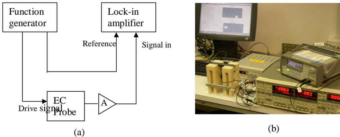
Fig. 1 Multi-frequency eddy current system for case depth measurement (a) diagram (b)
