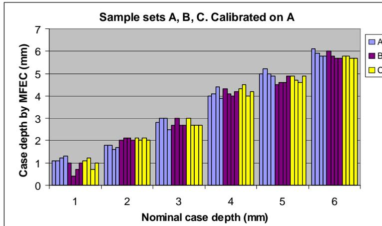
Fig. 6. Case depths measured with MFEC system for all the three sample sets.
