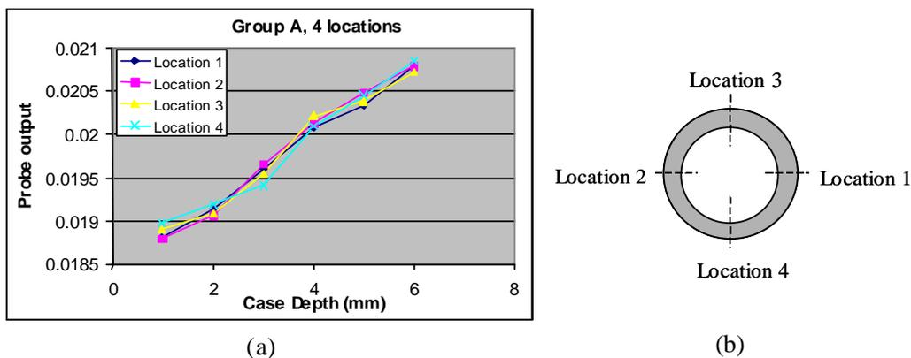
Fig. 5 (a) MFEC results on one set of samples at four locations along circumferential direction (b) illustration of four locations.
