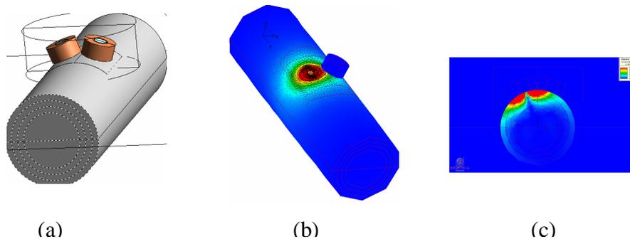
Fig. 3. FEM simulation for the circumferential probe. (a) FEM model (b) 3D view of eddy current field. (c) Cross section view of eddy current field in the sample.
