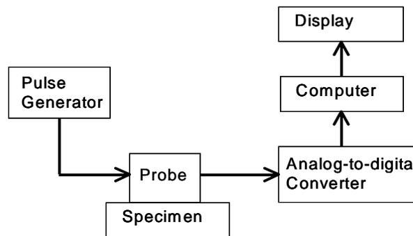
Fig. 2. Block diagram of the PEC system for case depth experimental setup
