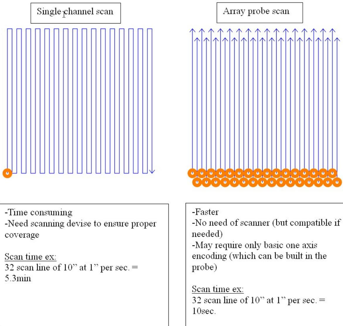
Arrays have been made from conventional coils and are therefore subject to the same limitations of single channel coils. Cost to manufacture can be significant. If a standard single channel pencil main cost is the manufacture of the coil itself, than a multi coil sensor will have incrementally greater cost of manufacture, which limits the range of applications where this technology can be economically used.
