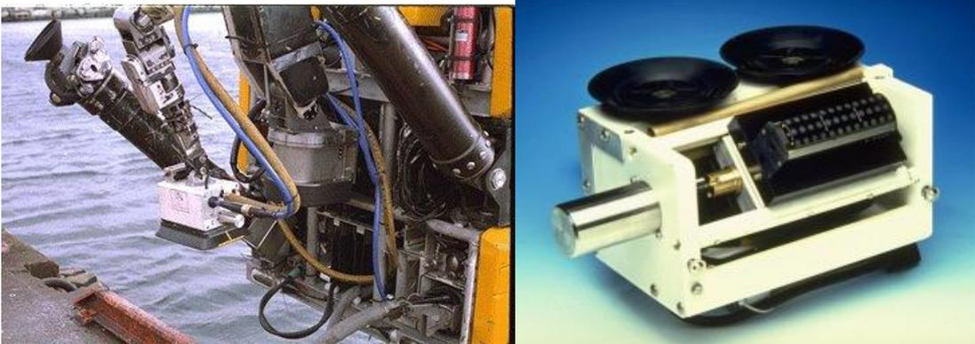
Figure 3. ACFM array probe for butt welds mounted on ROV (left); probe for fillet welds (right)
