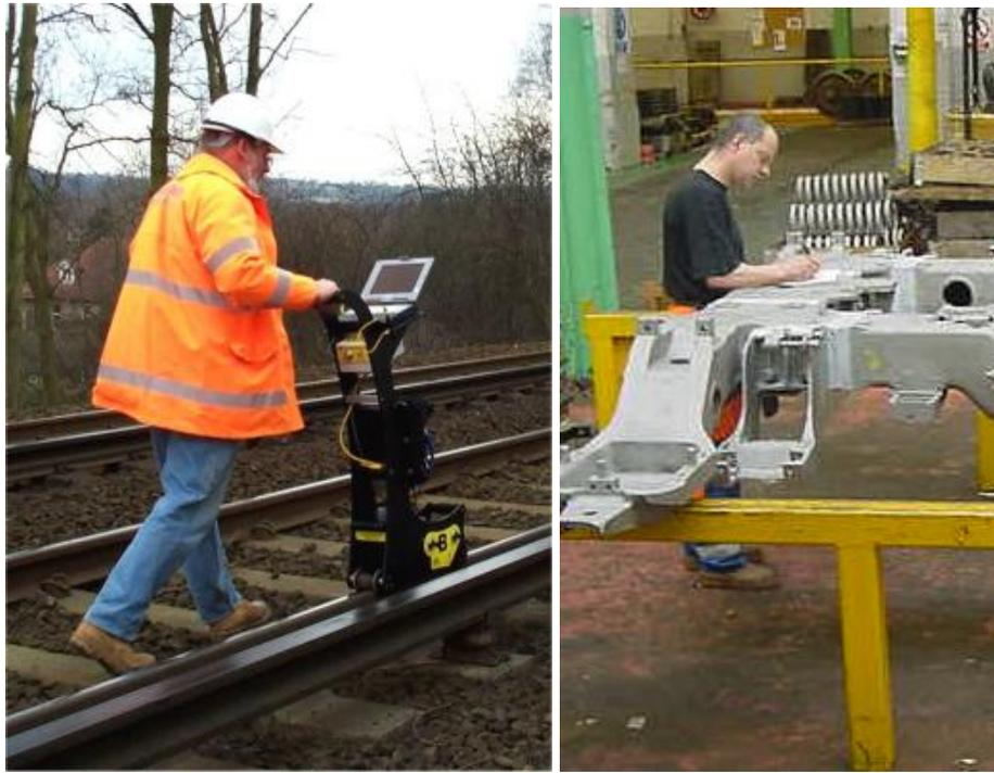
Figure 6. ACFM inspection of rails (left) and bogies (right)
