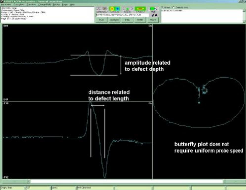
Figure 2. Typical ACFM signal response to a defect
