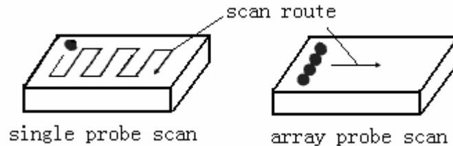
Fig 1 Schematic of single probe and array probe scan
