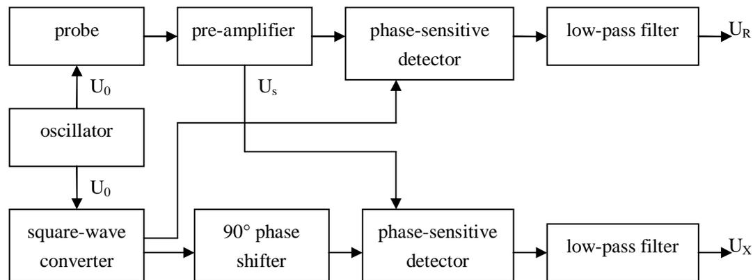
Fig 3 Schematic of X-R resolver
