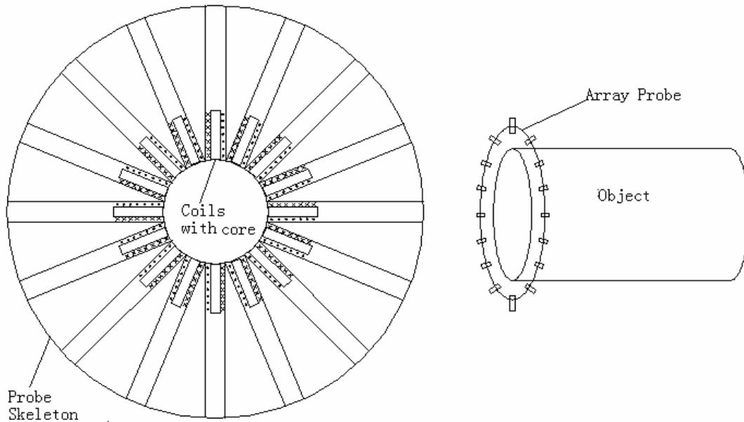
Fig 6 Schematic of array probe
