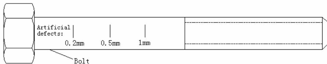
Fig 7 Schematic of artificial defects
