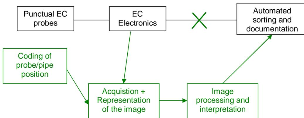
**Figure 3: The items shown in green need to be added to the current system for implementing the proposed solution**
