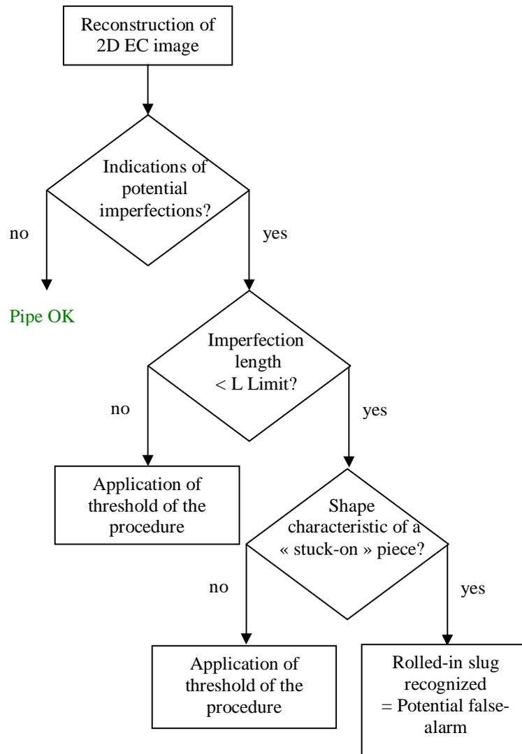
**Figure 2: The algorithm for recognizing rolled-in slug type flaws proceeds in three successive stages which make it possible to only confirm the presence of a rolled-in slug when it is certain of the type of flaw.**
