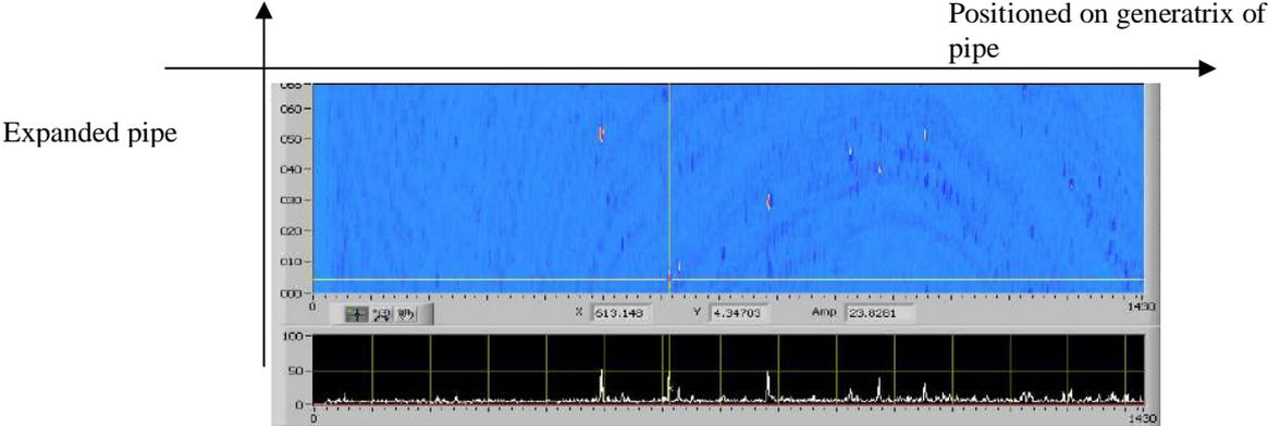
**Figure 1: Representation of the expanded EC image of the pipe compared with the conventional recording below.**
