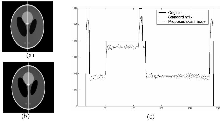
Figure 2 Slice at position  $z = -0.25$ . (a) Image reconstructed by using standard helix with large detector, (b) Image reconstructed by using proposed scan mode with small detector, (c) Profile on the line in left image.
