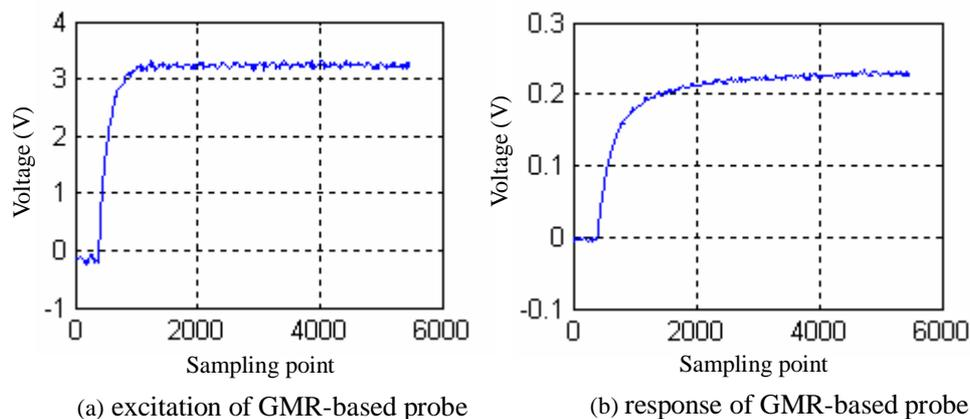
Fig.3 Excitation and response of GMR-based probe on 2mm specimen
