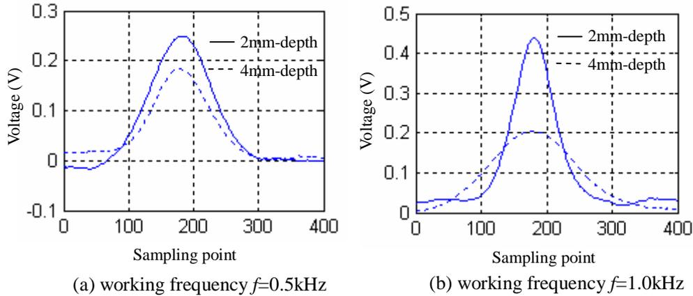
Fig.5 Signals for subsurface slots: 2mm-depth and 4mm-depth.
