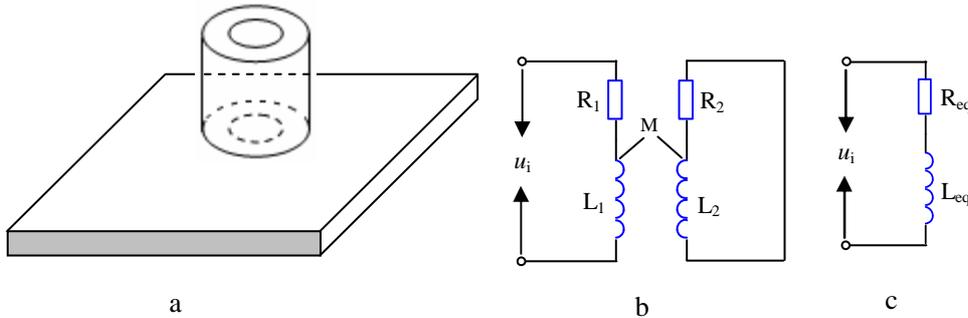
Fig.1. Probe-specimen setup and its equivalent circuit
