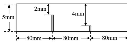
Fig.4 View of test sample and subsurface slots
