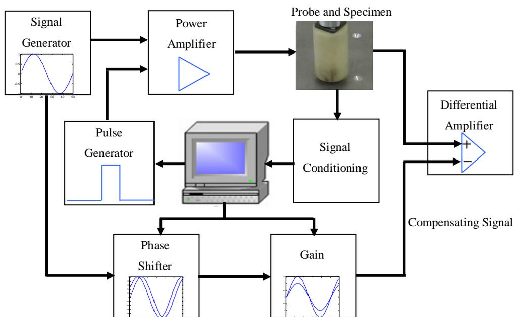
Fig.2 Schematic diagram of self-compensating GMR-based probe
