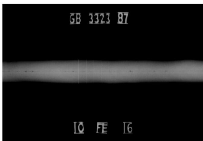
Diagram 1      Steel wire image quality indicator measures welding gap detection image quality
