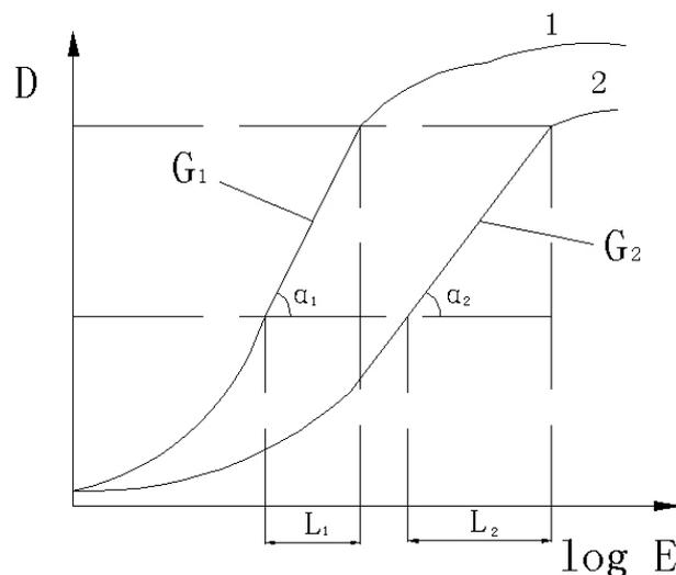
Diagram 2 Film property curve and tolerance
