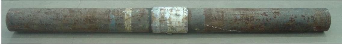
**Figure 2. Casing with coupling**
