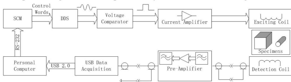
**Figure 1. PEC system setup**
