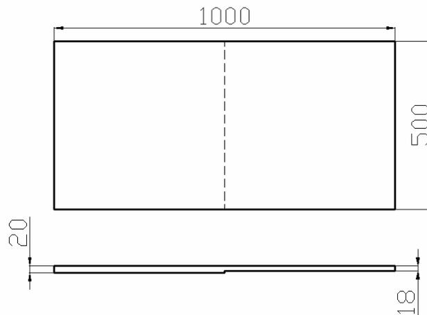
Figure 7. Dimension of two step wedge plate
