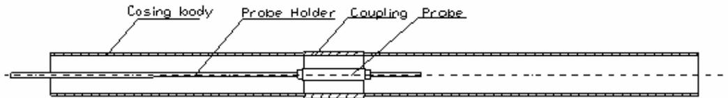
**(a) Internal testing of coupling**
