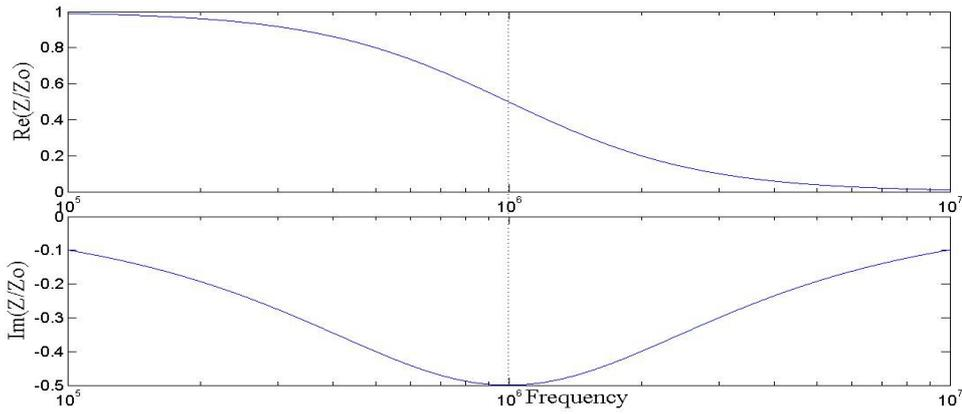
Fig.5 Analytic inductance of coil above a conductive plate
