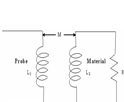
Fig.2 Circuit model for the eddy-current
