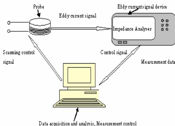
Fig.3 Basic eddy current testing system
