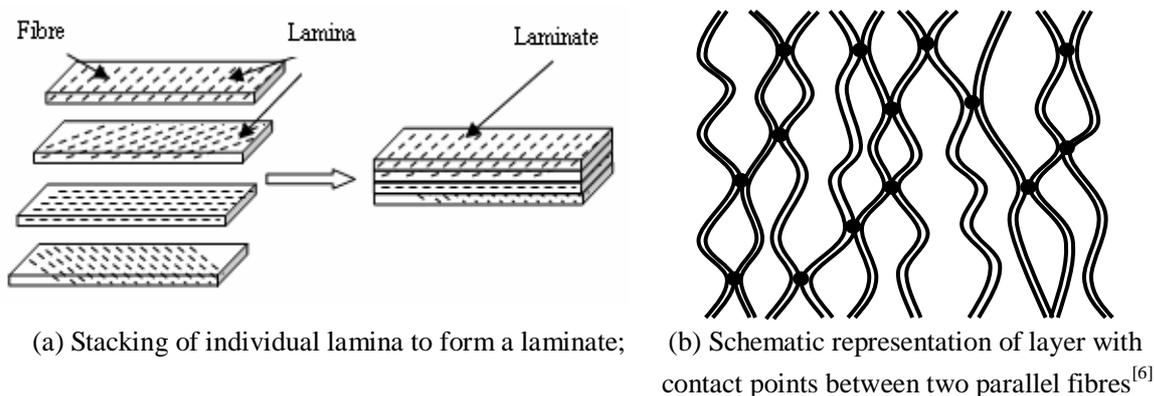
Fig.1 Formation and structure of CFRP composite
