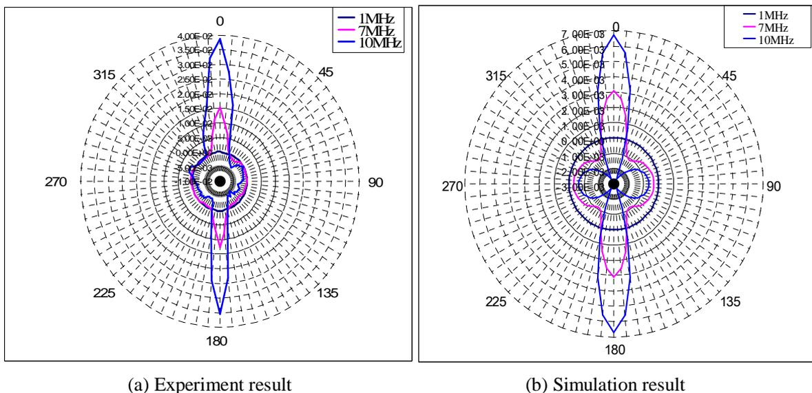
Fig.9 Results of fibre direction detection
