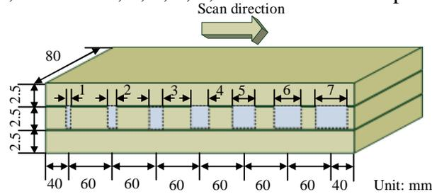
Fig.1 The sketch of defects of varying diameter in multi-layered structures (specimen #1).
