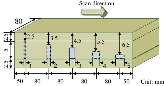
Fig. 3 The sketch of defects of varying diameter and depth in multi-layered structures (specimen #2).
